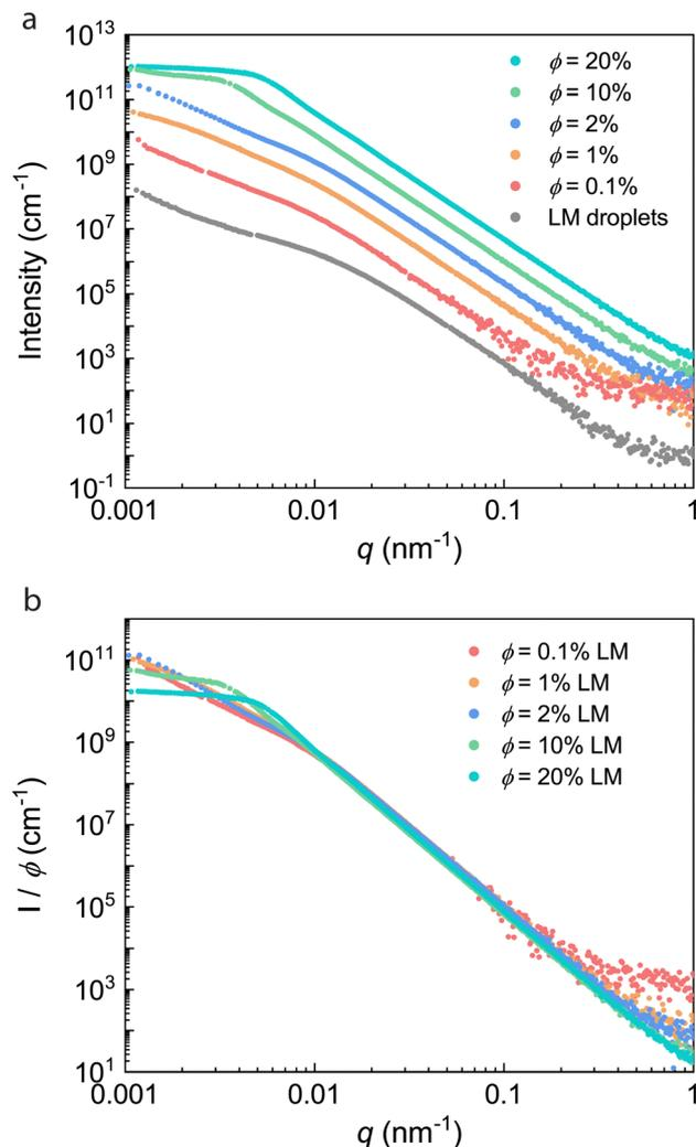
**Fig. 3** X-ray scattering curves. (a) Desmeared USAXS profiles of the LM droplets and composites at various LM loadings ( $\phi = 0.1, 1, 2, 10, 20\%$ ). The LM droplet profile is on the original scale and all other profiles are vertically offset for clarity. (b) Reduced scattering curves normalized for the volume loading  $\phi$  of the liquid metal filler.
