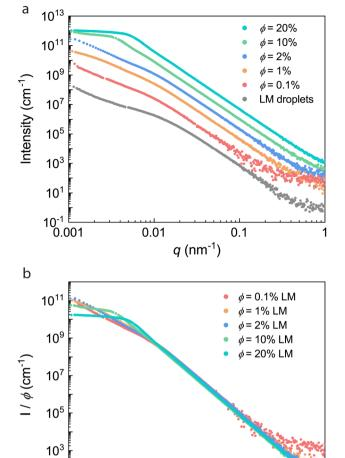
Fig. 3 X-ray scattering curves. (a) Desmeared USAXS profiles of the LM droplets and composites at various LM loadings ( $\phi$  = 0.1, 1, 2, 10, 20%). The LM droplet profile is on the original scale and all other profiles are vertically offset for clarity. (b) Reduced scattering curves normalized for the volume loading  $\phi$  of the liquid metal filler.
