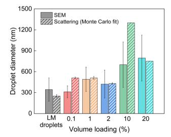
Droplet sizes for the pristine LM droplets and when dispersed as a Fig. 7 filler in PDMS at different volume loadings, as determined from the image analysis on SEM micrographs and Monte Carlo fits on the X-ray scattering data. The values from the Monte Carlo fit correspond to the particle size in the greatest frequency (i.e., the mode).
