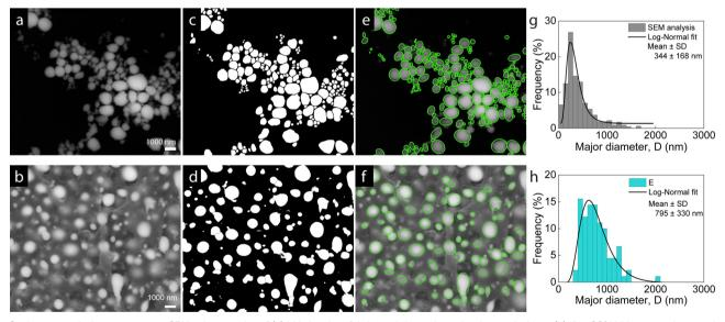
Fig. 2 Image analysis sequence on SEM micrographs of (a) LM droplets fabricated through sonication technique. (b)  $\phi = 20\%$  LM composites made by dispersing the droplets in PDMS. (c) and (d) Binary masks generated from the SEM images in (a) and (b). (e) and (f) Ellipses fit to the bright droplet areas in (c) and (d) and overlaid on the actual image, (g) and (h) major diameter of the ellipses in (e) and (f) are plotted to obtain histograms and mean size using a log-normal fit.
