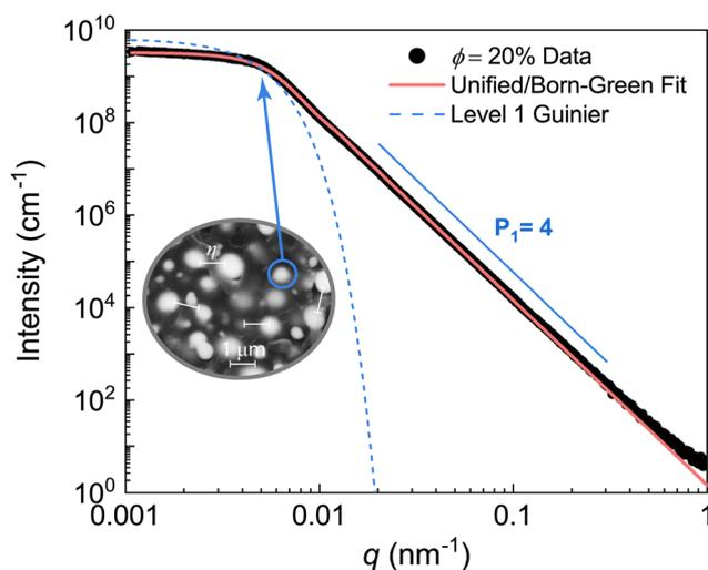
**Fig. 5** Unified fit of  $\phi = 20\%$  LM composite. The single structural level represents scattering from the primary droplets. The correlation length calculated from the Unified/Born–Green equation is on the order of 1  $\mu\text{m}$ . The fit parameters can be found in Table 2.
