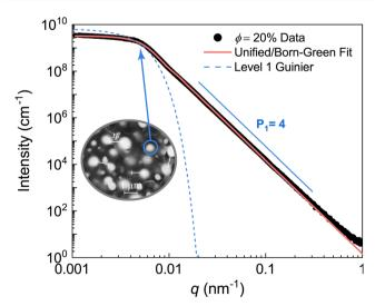
Fig. 5 Unified fit of  $\phi$  = 20% LM composite. The single structural level represents scattering from the primary droplets. The correlation length calculated from the Unified/Born-Green equation is on the order of 1  $\mu$ m. The fit parameters can be found in Table 2.
