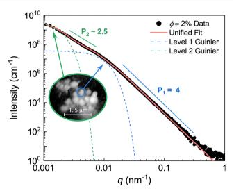
Fig. 4 Two-level Unified fit of  $\phi$  = 2% LM composite. Structural level 1 represents scattering from the primary droplets, and structural level 2 represents scattering from the mass-fractal LM aggregates. The fit parameters can be found in Table 1.
