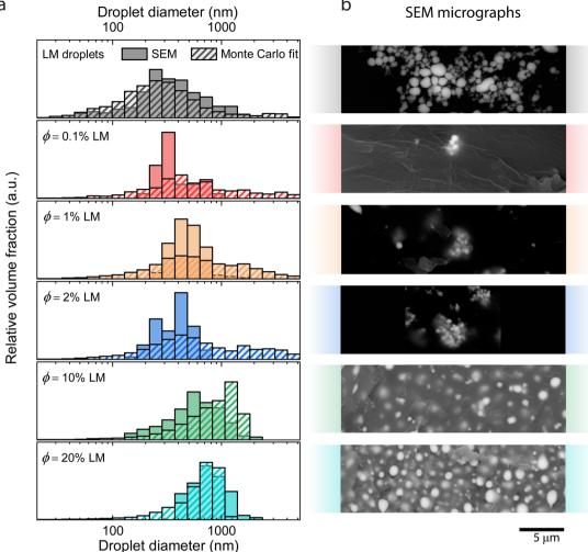
Fig. 8 (a) Size distributions of the LM droplets and composites at various LM loadings ( $\phi = 0.1, 1, 2, 10, 20\%$ ) overlaid on the histrograms obtained from Monte Carlo fits on the scattering data. (b) Representative SEM micrographs of the samples corresponding to the histogram overlays. The histograms have been normalized such that the total area of all bins is equal to 100%.
