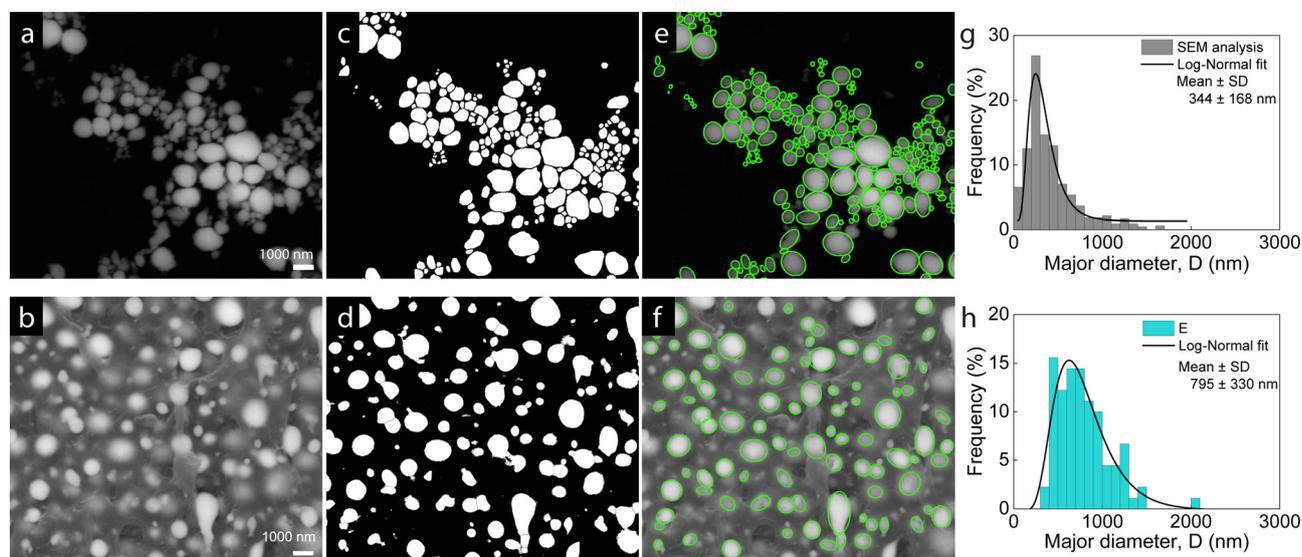
Fig. 2 Image analysis sequence on SEM micrographs of (a) LM droplets fabricated through sonication technique. (b)  $\phi = 20\%$  LM composites made by dispersing the droplets in PDMS. (c) and (d) Binary masks generated from the SEM images in (a) and (b). (e) and (f) Ellipses fit to the bright droplet areas in (c) and (d) and overlaid on the actual image, (g) and (h) major diameter of the ellipses in (e) and (f) are plotted to obtain histograms and mean size using a log-normal fit.
