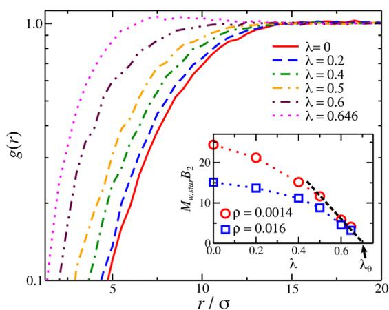
Fig. 7 Pair correlation function,  $g(r)$ , for center of mass star polymer ( $f = 4$  arms and  $M = 25$  arm length) solution at a segmental density  $\rho\sigma^3 \approx 0.016$ . Inset: Second virial of star polymer solutions as a function of  $\lambda$ ; results at different polymer concentrations are also presented. The dashed line is an extrapolation to identify the  $\theta$ -point at  $B_2 = 0$ .
