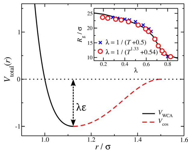
**Fig. 1** The non-bonded, bead–bead interaction potential  $V(r)$  with  $\lambda = 1$ , showing the contributions from  $V_{WCA}(r) + V_{SW}(r)$  (black) and  $V_{cos}(r)$  (red). Inset: Average radius of gyration of a nanogel particle *via*  $\lambda$  variation (black line) and temperature  $T$  variation (symbols). Two relations between  $\lambda$  and  $T$  are presented.
