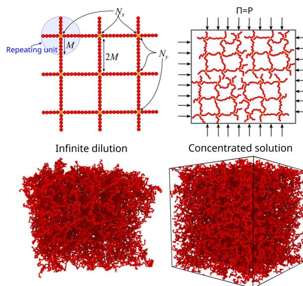
**Fig. 2** Schematic of the molecular architecture of the nanogel particle. Typical screenshots of an equilibrated molecular configuration of compact nanogel particle at infinite dilution (the simulation box is so large that is not visible) and fixed osmotic pressure conditions, where the nanogel particles fill the simulation box and interacting through periodic boundaries.
