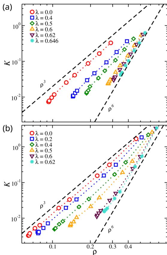
Fig. 10 Osmotic modulus,  $K$ , of compact nanogel particles as a function of segmental density,  $\rho$ . Results for different solvent qualities are also presented. The dashed lines are guides for the eye.
