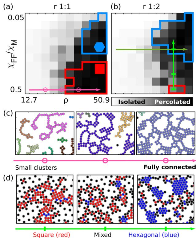
Fig. 4 The percolated, hexagonal and square phases plotted over interaction and density for ratios  $r = 1:1$  (a) and  $r = 1:2$  (b). (c) The transition from isolated beads to percolated with increasing bead density for  $r = 1:1$ . (d) The transition from square to hexagonal configuration with varying interactions for  $r = 1:2$ .
