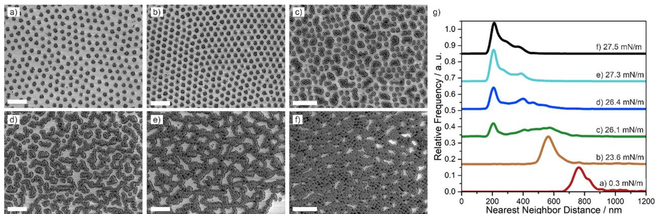
**Fig. 3** Interfacial phase behavior of 198 nm–10 mol% core–shell particles. (a)–(f) SEM images taken after deposition to a solid substrate from the air/water interface at different surface pressures. (g) Corresponding nearest neighbor distributions. The particles undergo a phase transition from hexagonal non-close packed arrangements (a) and (b) to chain-like networks (d) and (e) to a dense chain network (f) upon compression. Scale bar: 2  $\mu\text{m}$ .
