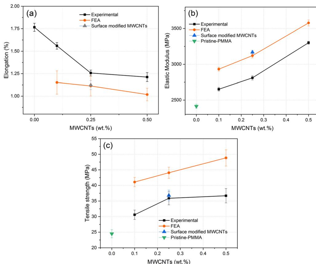
Fig. 8 Variation of experimental and FEA values of (a) % elongation, (b) EM, and (c) TS with the content of MWCNTs in the PMMA matrix.
