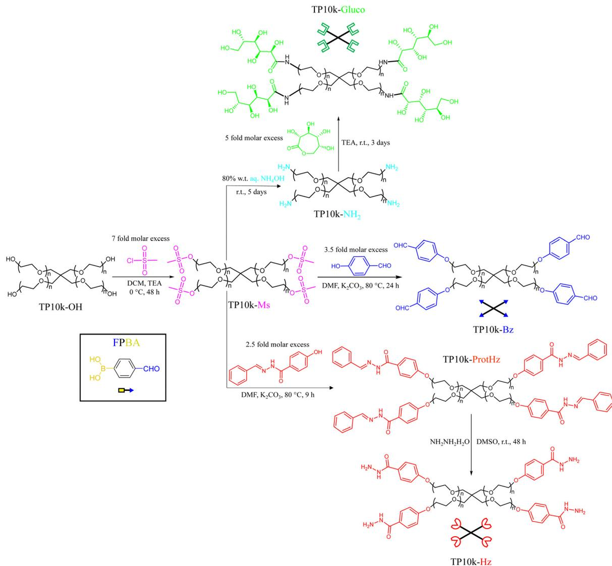
Fig. 1 Reaction schemes followed for the preparation of the three differently end-functionalized tetraPEGs, as well as their schematic representations plus that of FPBA.
