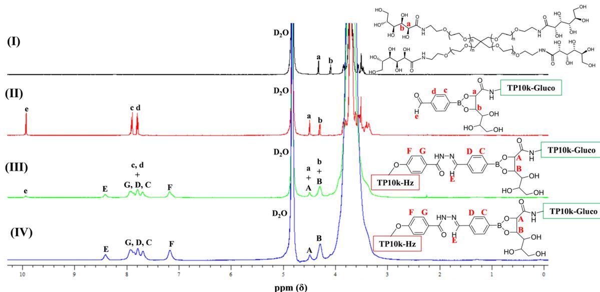
Fig. 4  $^1\text{H}$  NMR spectra in  $\text{D}_2\text{O}$  buffered at  $\text{pD} = 8.5$  of (I) the starting TP10k-Gluco, (II) the fully-formed (within 1 h) adduct of TP10k-Gluco with a stoichiometric amount of FPBA, and (III and IV) the “boronate” hydrogel formed from the reaction of the TP10k-Gluco-FPBA adduct with a stoichiometric amount of TP10k-Hz after three days (III) and after seven (IV).
