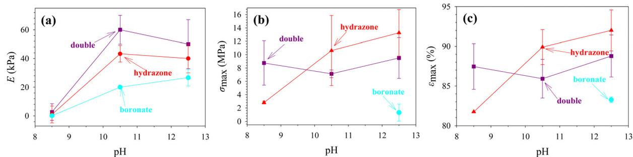
Fig. 10 Compressive mechanical properties, (a) elastic modulus,  $E$ , (b) stress at break,  $\sigma_{max}$ , and (c) strain at break,  $\epsilon_{max}$ , of the three hydrogel types, boronate, hydrazone and double, each prepared at three different pH values, 8.5, 10.5 and 12.5.
