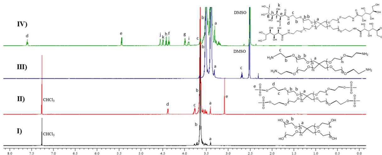
Fig. 2  $^1\text{H}$  NMR spectra of (I) the starting compound TP10k-OH, (II) the purified mesylate-terminated tetraPEG (TP10k-mesyl), (III) the purified amine-terminated tetraPEG (TP10k-NH<sub>2</sub>), and (IV) the final targeted product of diol-terminated tetraPEG (TP10k-Gluco).
