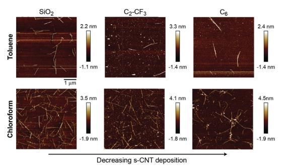
Fig. 4 Representative atomic force microscopy images of PFO-BPy-wrapped s-CNTs deposited on bare SiO<sub>2</sub> or surfaces grafted with C<sub>2</sub>-CF<sub>3</sub> or C<sub>6</sub> SAMs. Deposition was quantified for  $2 \mu g \, mL^{-1} \, s$ -CNTs in either toluene (top row) and chloroform (bottom row) ink. s-CNTs are visible as thin white lines in the AFM images.
