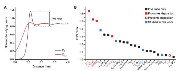
Fig. 2 A Toluene density profile near the  $C_2$ -grafted surface (black) and the  $C_{22}$ -grafted surface (red). The first peak of the red curve was shifted to overlap with that of the black curve to help compare differences in peak: well ratios. B Peak: well (P:W) ratios for all SAM-grafted surfaces. Surfaces shown to promote (filled red) or prevent (hollow red) s-CNT deposition in past work are indicated.<sup>25</sup> Blue squares indicate SAMs selected for additional study in this work
