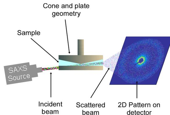
**Fig. 1** Schematic of the RheoSAXS setup where X-ray the beam passed through a hole at the bottom plate at a  $5^\circ$  angle and then through the sample capturing the scattering data in the 1–2 plane.
