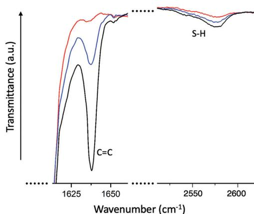
Fig. 3 FTIR signatures of transmission peaks of  $\text{-SH}$  and of  $\text{-C=C}$  bonds in the reacting mixture (in this case, for the RM105 elastomer reaction). The curves are for  $t = 0$  (for which, as a model, we used the reacting mixture without catalyst), for 5 minutes, and for 3 hours of reaction. The acrylate peak disappears completely in 3 hours, confirming the completion of the reaction. The thiol peak does not disappear completely, which is a known feature.<sup>27,28</sup>
