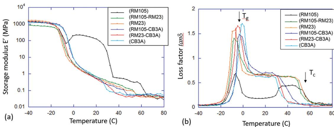
**Fig. 5** Dynamic mechanical analysis of xLCE. (a) The linear storage modulus  $E'$  (a) and the loss factor  $\tan\delta$  (b) measured at a constant frequency of 1 Hz, are plotted against temperature. The curves are marked by the mesogen species in each sample: CB3A; RM105; RM23; RM105 + RM23; RM105 + CB3A; and RM23 + CB3A. The arrows indicate the glass and the isotropic transition points that have a very clear signature in the DMA signal.
