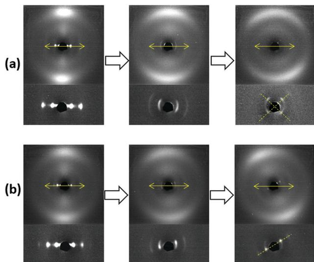
Fig. 7 XRD patterns of aligned samples synthesized from (a) RM105 and (b) RM105 + RM23, with the increasing degree of stretching from left to right (starting with no stretching). The stretching direction along the nematic director and the layer normal is marked on all wide-angle XRD patterns by double-headed arrows. In the last stage of stretching, the diagonals on which smectic-layer signals reside are marked by dashed lines.
