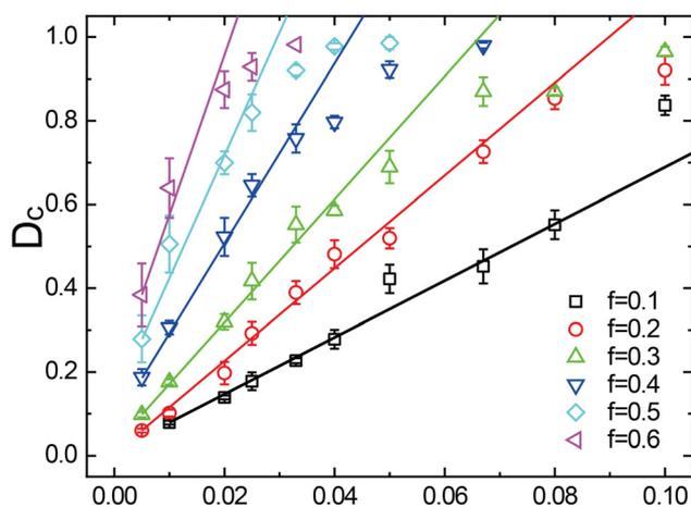
Fig. 4 Duty cycle of NPDs through nanochannels as a function of incident flow rate and at different drift forces. MD simulation results (symbols) display a linear relationship between  $D_c$  and  $I$  (solid lines, eqn (6)), which fails as  $D_c$  approaches 1.
