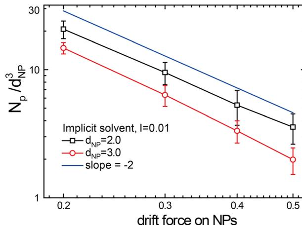
Fig. 6 The average number of NPs inside a "droplet",  $N_p$ , as a function of drift force,  $f$ . Black and red symbols represent free NP diameters of  $d_{NP} = 2$  and  $d_{NP} = 3$ , respectively, and the simulation results for both are consistent with the prediction of the scaling relation  $N_p \sim f^{-2}$  (eqn (5), blue line) within the error range.
