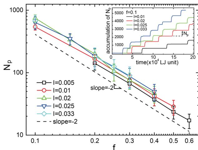
Fig. 2 The average number of nanoparticles inside a NPD,  $N_p$ , as a function of drift force,  $f$ . Symbols of different colors represent simulations at different incident rates. The dashed line is the slope  $s = -2$  according to the scaling relation eqn (5). Inset: Stepwise accumulation of nanoparticles arriving at the sink area at different production rates but constant driving force.
