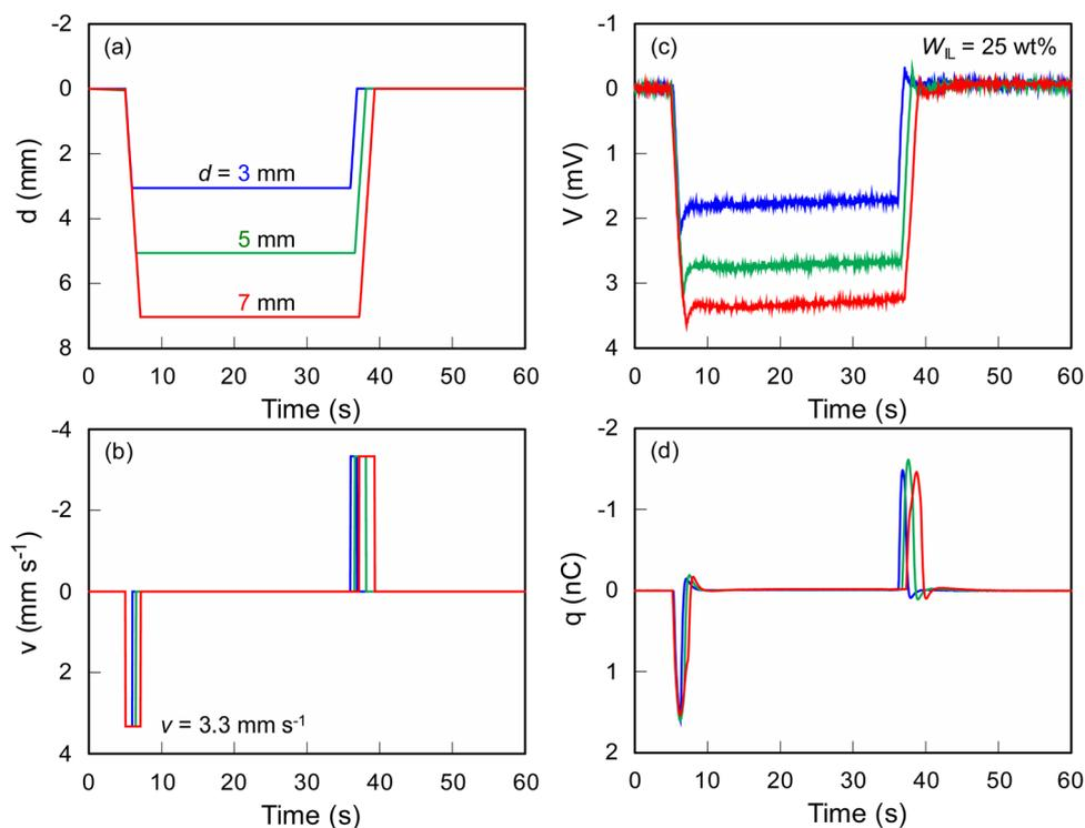
Fig. 7 Relation between input mechanical stimuli of (a) constant bending velocity ( $v = 3.3 \text{ mm s}^{-1}$ ) with (b) different displacements ( $d = 3, 5, 7 \text{ mm}$ ) and output electric signals of (c) voltage ( $V$ ) and (d) electric charge ( $q$ ) of ionic SMP gel sensor ( $W_{IL} = 25 \text{ wt\%}$ ).
