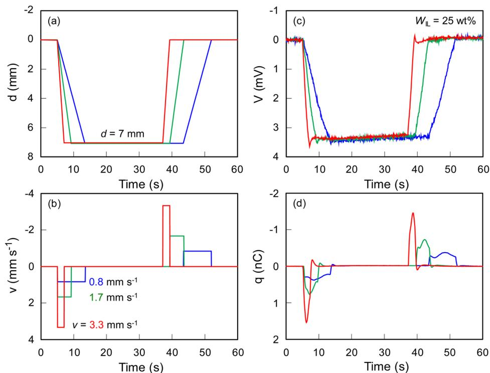
Fig. 6 Relation between input mechanical stimuli of (a) constant bending displacement ( $d = 7 \text{ mm}$ ) with (b) different velocities ( $v = 0.8, 1.7,$  and  $3.3 \text{ mm s}^{-1}$ ) and output electric signals of (c) voltage ( $V$ ) and (d) electric charge ( $q$ ) of ionic SMP gel sensor ( $W_{IL} = 25 \text{ wt\%}$ ).
