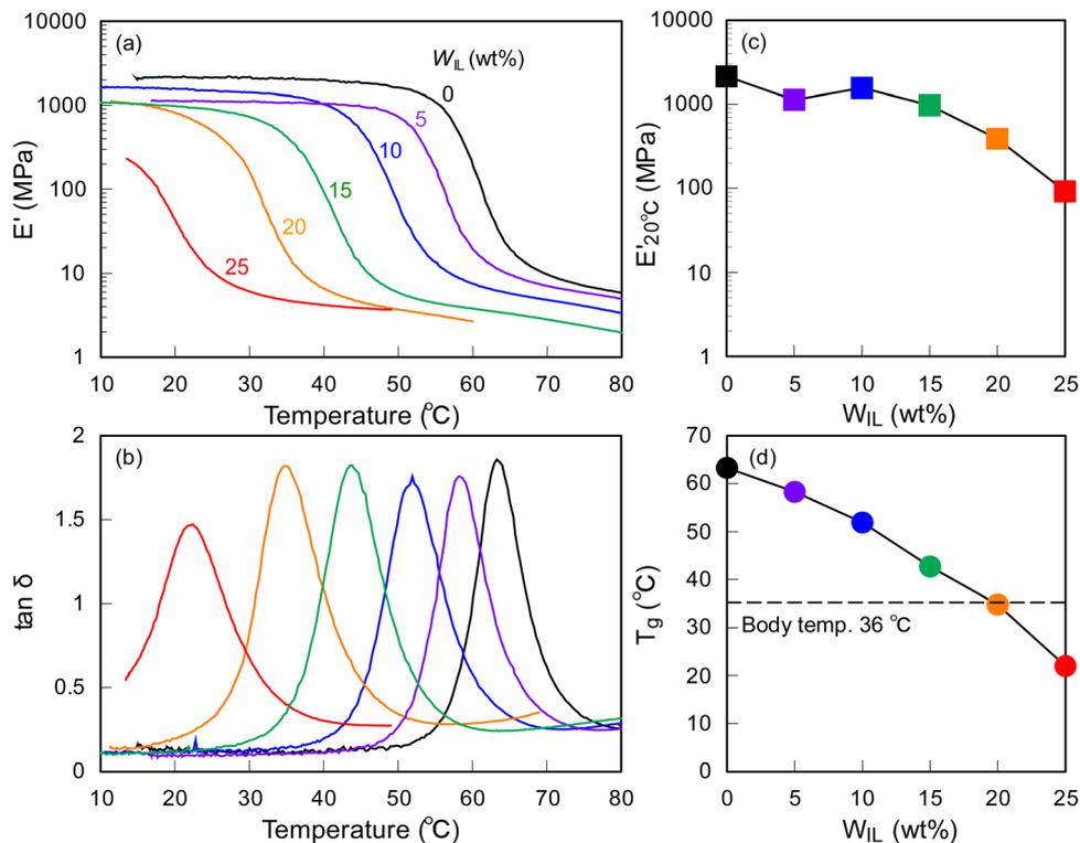
Fig. 2 Temperature dependence of (a) storage modulus ( $E'$ ) and (b) loss tangent ( $\tan \delta$ ) for ionic SMP gels with different  $W_{IL}$ . Dependence of (c) storage modulus at 20 °C ( $E'_{20^\circ\text{C}}$ ) and (d)  $T_g$  of ionic SMP gels on  $W_{IL}$ .
