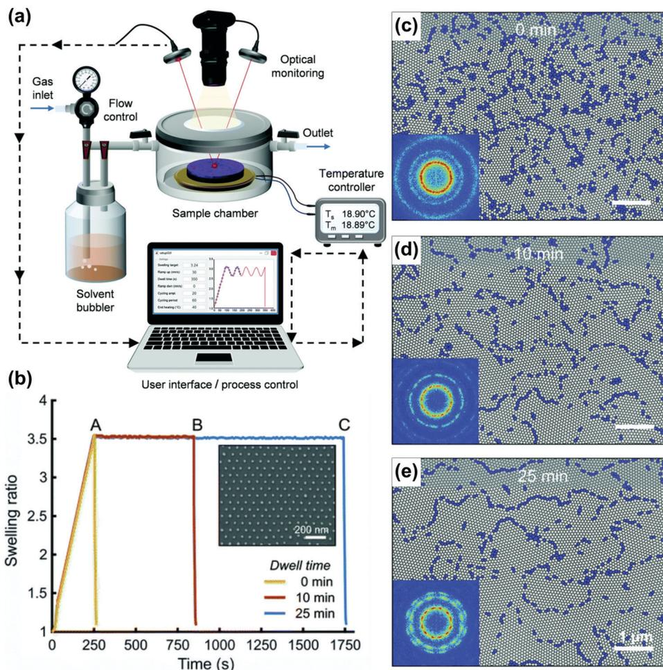
Fig. 8 Automated solvent vapor annealing. (a) Schematic of an advanced SVA setup with closed-loop SR control. (b) Annealing pathways of cylinder-forming PS-*b*-P2VP 258 kg mol<sup>-1</sup> thin films in THF vapor and corresponding morphologies after 0, 10, and 25 min (c–e). Adapted from *Soft Matter*, **15**, 7909.<sup>176</sup> With permission from The Royal Society of Chemistry.
