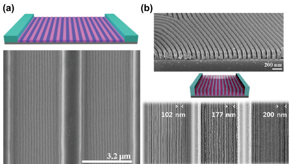
**Fig. 11** Solvent vapor-assisted graphoepitaxial ordering of high MW PS-*b*-PMMA lamellar patterns. SEM images of films in trench confinement. (a) 3.2  $\mu\text{m}$  wide trench; (b) cross-section view and top-down images of 1.5  $\mu\text{m}$  wide trench. Reprinted with permission from *Macromolecules*, **49**, 1722,<sup>88</sup> and *ACS Nano*, **7**, 1952.<sup>159</sup> Copyright 2016, 2013 American Chemical Society.
