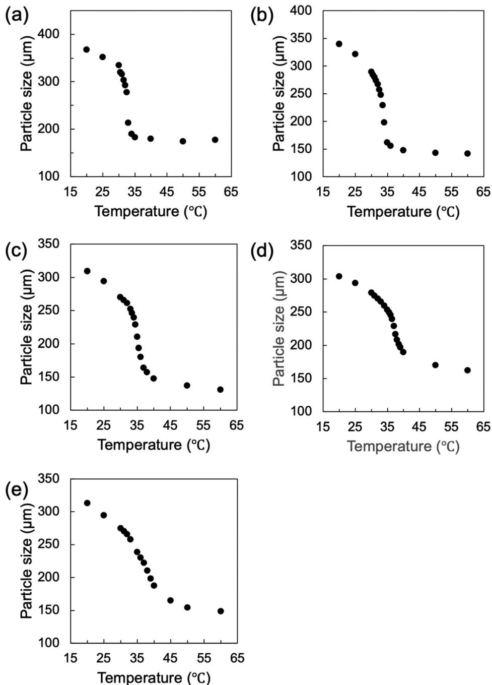
Fig. 6 Diameter of the spherical gels (a) PNIPAA gel, (b) PNIPAA<sub>0.9</sub>-*b*-PDMA<sub>0.1</sub> gel, (c) PNIPAA<sub>0.8</sub>-*b*-PDMA<sub>0.2</sub> gel, (d) PNIPAA<sub>0.7</sub>-*b*-PDMA<sub>0.3</sub> gel and (e) PNIPAA<sub>0.8</sub>-*r*-PDMA<sub>0.2</sub> gel at equilibrium at certain temperature for each of them. The diameters are measured through an inverted optical microscope.
