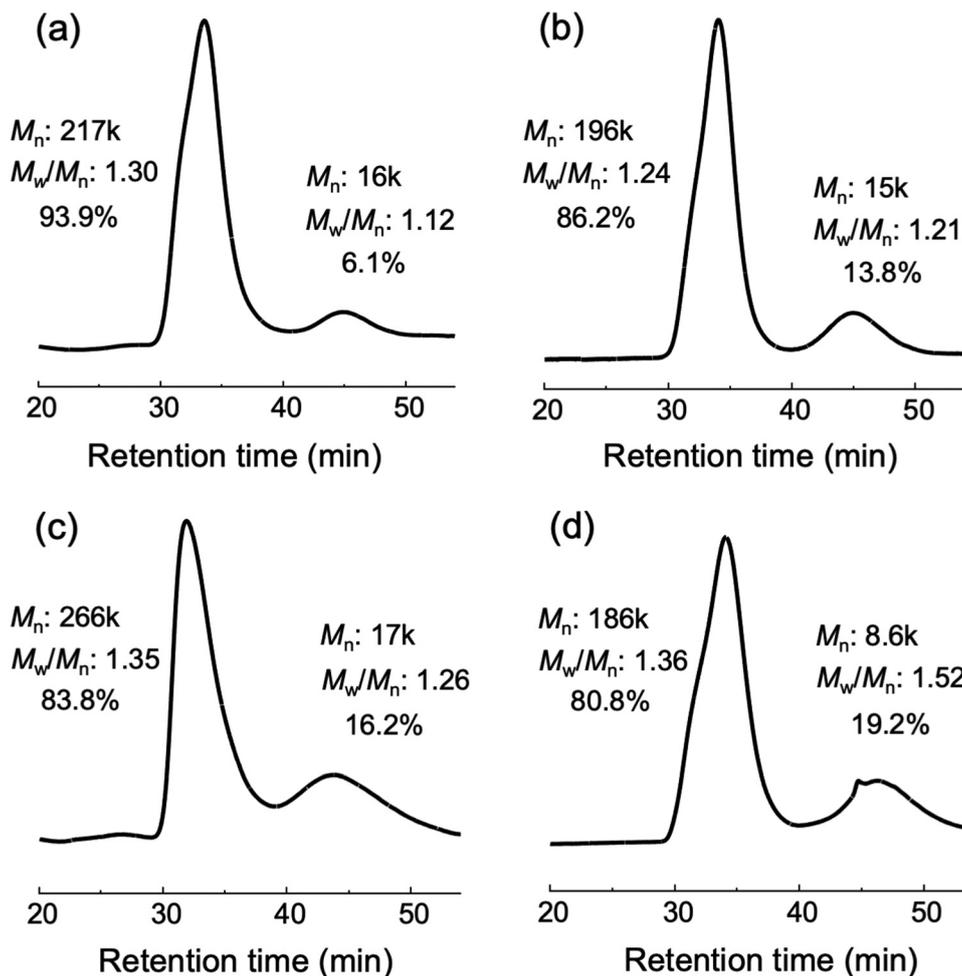
Fig. 4 SEC curve obtained after methanolysis decomposition of (a) PNIPA gel, (b) PNIPAA<sub>0.9</sub>-*b*-PDMA<sub>0.1</sub> gel, (c) PNIPAA<sub>0.8</sub>-*b*-PDMA<sub>0.2</sub> gel and (d) PNIPAA<sub>0.7</sub>-*b*-PDMA<sub>0.3</sub> gel.
