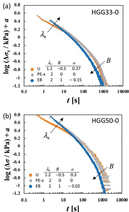
Fig. 5 Failure of the superposition of  $\log \Delta\sigma - \log t$  curves for different types of deformation with various values of  $\lambda_x$  by vertical shift with a factor of  $a$  for (a) HGG33-0 and (b) HGG50-0. Qualitative features of the failure of the superposition are common to HGG33-0, HGG50-0 and HGG64-0 (Fig. 4).
