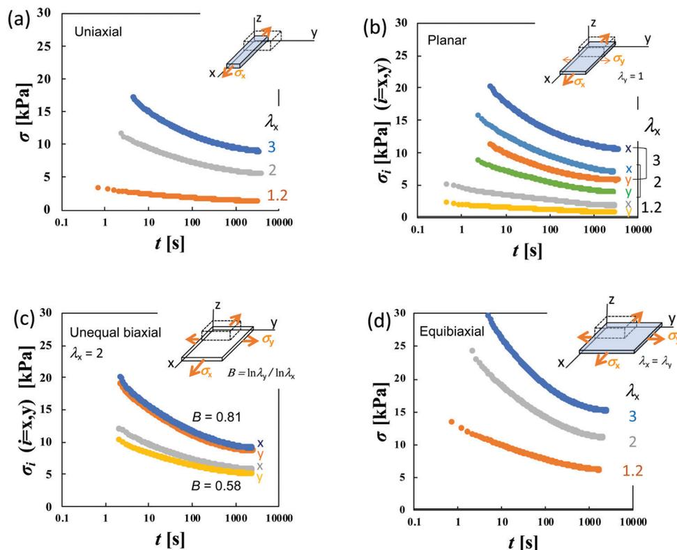
Fig. 3 Elapsed time ( $t$ ) dependence of nominal stress ( $\sigma$ ) for HGG63-0 after the imposition of (a) uniaxial, (b) planar, (c) unequal biaxial and (d) equibiaxial extension with various degrees of imposed stretching.
