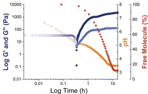
Fig. 5 Time sweep analysis for DTDPP-A-OH with  $G'$  (dark blue),  $G''$  (light blue), pH (orange) and % free molecule by NMR spectroscopy (dark red) shown with time as the gelation occurs after GdL addition.
