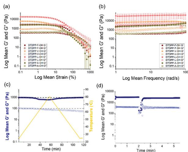
**Fig. 4** (a) Strain and (b) frequency sweeps for DTDPP-F-OH 5 mg mL<sup>-1</sup>, DTDPP-V-OH 10 mg mL<sup>-1</sup>, DTDPP-L-OH 15 mg mL<sup>-1</sup>, and DTDPP-A-OH 5 mg mL<sup>-1</sup>. (c) Temperature sweep for DTDPP-F-OH 5 mg mL<sup>-1</sup> gel showing  $G'$  (dark blue) and  $G''$  (light blue), and temperature (yellow) and (d) thixotropy sweep for DTDPP-F-OH 5 mg mL<sup>-1</sup> gel showing  $G'$  (dark blue) and  $G''$  (light blue).
