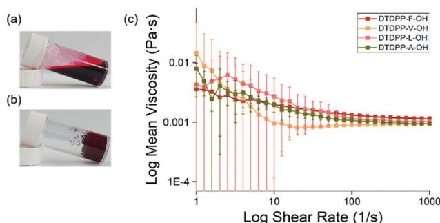
**Fig. 3** (a) DTDPP-V-OH pH 10.5 sol (b) DTDPP-V-OH gel (c) viscosity measurements for DTDPP-F-OH 5 mg mL<sup>-1</sup>, DTDPP-V-OH 10 mg mL<sup>-1</sup>, DTDPP-L-OH 15 mg mL<sup>-1</sup>, and DPP-A-OH 5 mg mL<sup>-1</sup> (all in water at pH 10.5).
