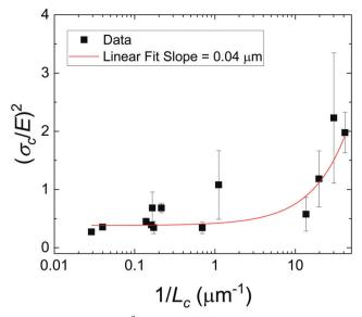
Fig. 5 Plot showing  $(\sigma_c/E)^2$  against  $1/L_c$  for the composite hydrogels used in this study. Note that the x-axis is plotted in log scale. The slope on this plot, 0.04 µm, is well below the elastofracture length of these materials and no significant transition is observed. This likely indicates that the assumption that  $a = L_c$  in the absence of a macroscopic notch is incorrect.
