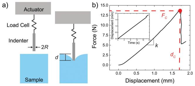
Fig. 2 (a) Sketch of the deep indentation and puncture measurements. (b) Plot of the force displacement curve with the critical puncture force and displacement marked in red. The inset graph shows the displacement vs time profile.
