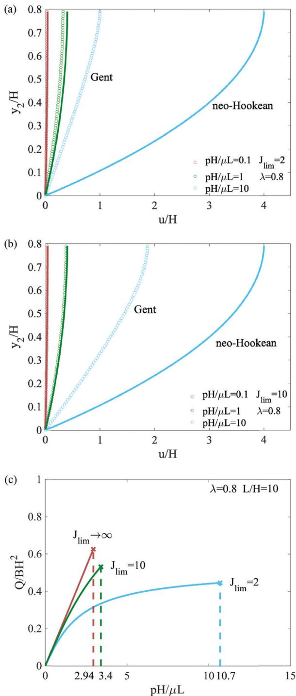
Fig. 4 (a and b) Displacement of seals for both strain-stiffening (open circle) and neo-Hookean (solid line) materials under different fluid pressures. (c) Relation between the fluid pressure  $p$  and the extrusion volume  $Q$ , plotted in the dimensionless form for both strain-stiffening ( $J_{\text{lim}} = 2, 10$ ) and neo-Hookean ( $J_{\text{lim}} \rightarrow \infty$ ) materials. Cross markers are critical points for seals to leak by elastic deformation.
