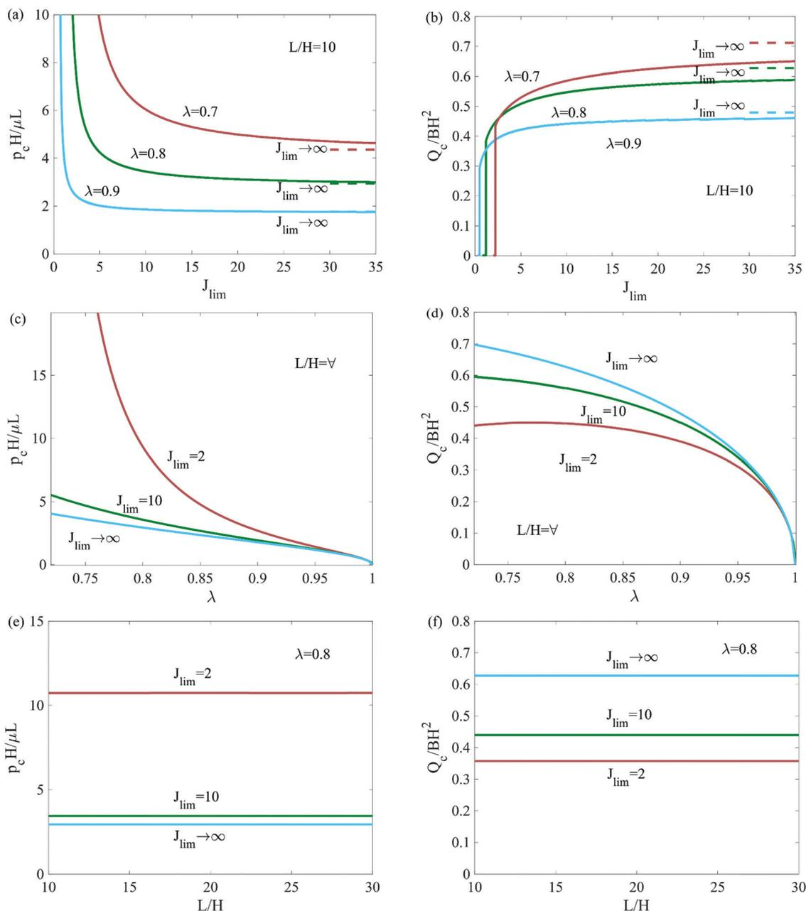
Fig. 5 The critical pressure  $p_c$  and extrusion volume  $Q_c$  for elastic leak as functions of  $J_{\text{lim}}$ ,  $\lambda$ , and  $L/H$ .
