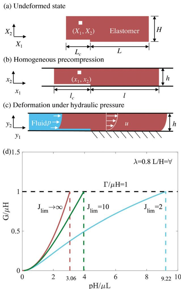
Fig. 6 A model of rupture. (a–c) The model assumes a debonded region of length  $l_c$  located at the bottom of the upstream front of the seal. (d) The relation between energy release rate  $G$  and pressure  $p$ . A strain-stiffening material will enhance the critical pressure of rupture compared to a neo-Hookean material.
