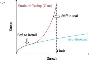
Fig. 1 Elastomeric seals. (a) An elastomer is precompressed between two rigid walls and is subject to fluid pressure. (b) Stress-stretch curves of a neo-Hookean material and a strain-stiffening material.
