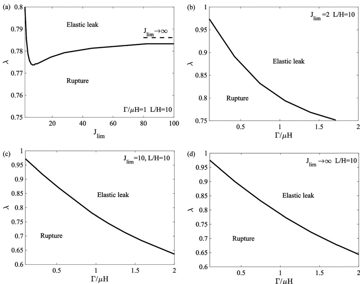
Fig. 8 Leak by elastic deformation and leak by rupture are demarcated on planes of various axes. (a) The diagram in the  $J_{\text{lim}}-\lambda$  plane for strain-stiffening seals with the fixed  $\Gamma/\mu H$  and  $L/H$ . (b) The diagrams in the  $\Gamma/\mu H-\lambda$  plane for strain-stiffening seals with the fixed  $J_{\text{lim}}$  and  $L/H$ . (c) The diagrams in the  $\Gamma/\mu H-\lambda$  plane for neo-Hookean seals with the fixed  $L/H$ .
