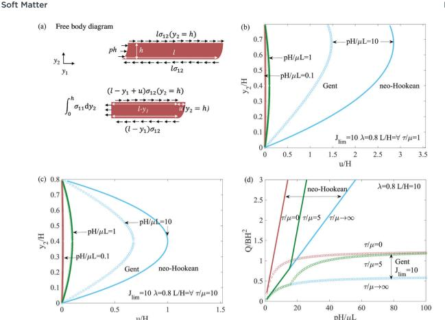
Fig. 9 (a) Free body diagram of the seal with friction at the top. (b and c) Displacement u of seal materials at height of  $y_2$ ,  $\tau/\mu$  is the dimensionless friction on the upper boundary. (d) p-Q curves for both strain-stiffening (Gent) and neo-Hookean seals when friction at the top surface of the seal is considered, assuming no leak happens.
