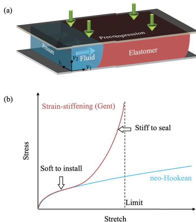
**Fig. 1** Elastomeric seals. (a) An elastomer is precompressed between two rigid walls and is subject to fluid pressure. (b) Stress–stretch curves of a neo-Hookean material and a strain-stiffening material.
