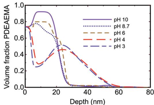
Fig. 3 Brush conformation as a function of pH for a PDEAEMA brush as obtained using neutron reflectometry.<sup>83</sup> The dry brush is 13 nm thick. The silicon substrate is equivalent to a volume fraction of 0.74.
