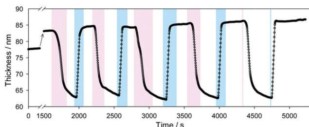
Fig. 4 The swelling and collapse of a PDEAEMA brush as an applied voltage across the brush is changed from +5 V (pink) to -5 V (blue). Figure reproduced with permission from the original article.<sup>98</sup> Copyright 2013 American Chemical Society.
