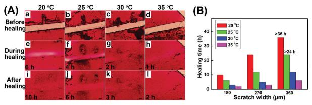
Fig. 6 (A) Microscope images of self-healing for hydrogel coatings under the temperature conditions of 20 °C, 25 °C, 30 °C, and 35 °C (scratch width: about 180  $\mu$ m, humidity: 40% RH, scale bar: 100  $\mu$ m). (B) Healing curves of hydrogel coatings with various scratch widths in different temperature conditions.
