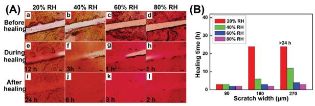
Fig. 7 (A) Microscope images of self-healing for hydrogel coatings under the humidity conditions of 20%, 40%, 60% and 80% (scratch width: about 180  $\mu$ m, temperature: 25 °C, scale bar: 100  $\mu$ m). (B) Healing curves of hydrogel coatings with various scratch widths in different humidity conditions.
