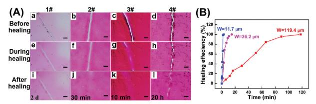
Fig. 5 (A) Microscope images of self-healing in ambient environments for hydrogel coatings with the corresponding experiment parameters in Table 1 (Scratch width: about 25 μm, scale bar: 100 μm). (B) Healing curves of hydrogel coatings (3# sample in Table 1) with different scratch widths of 11.7, 36.2 and 119.4 μm.
