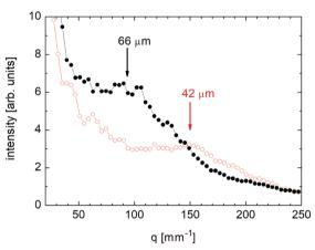
Fig. 8 Top: Contrast enhanced axial view of the central film of the catenoid in Fig. 5, 6 ms before pinch-off, image size  $6 \times 6$  mm<sup>2</sup>. Two regions with film thicknesses of 160  $\pm$  40 nm (left square in the image, filled symbols in the graph) and 90  $\pm$  40 nm (top right square in the image, open symbols) were cut out and Fourier transformed, yielding the spectra in the bottom graph.
