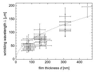
Fig. 9 Wavelengths determined in different collapse experiments in regions of nearly constant local film thickness d. The wavelengths were determined between 5 ms and 3 ms before the pinch-off, when the film had a diameter between 4 mm and 6 mm. The wave lengths could be determined with an accuracy of about 20%. The dashed line is a fit with  $\lambda = 0.25 \text{ m}^{1/2} \sqrt{d}$
