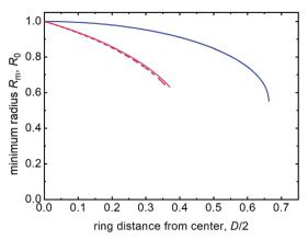
Fig. 2 Simple catenoid waist radius  $R_0$  (solid, blue) and central film radius of catenoids with middle membrane (dashed, red) as functions of the distances of the support rings from the catenoid center. The magenta curve is corrected for a potential negative line tension of the Plateau border (see text).  $R_0$ ,  $R_{\rm m}$  and D/2 are given in units of the ring radius R.
