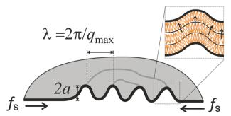
Fig. 11 Schematic drawing of the film wrinkles. The lateral forces  $f_s$ originate from the collapsing catenoid. The enlarged section sketches the smectic layers and mean orientation of molecules in a smectic A film.
