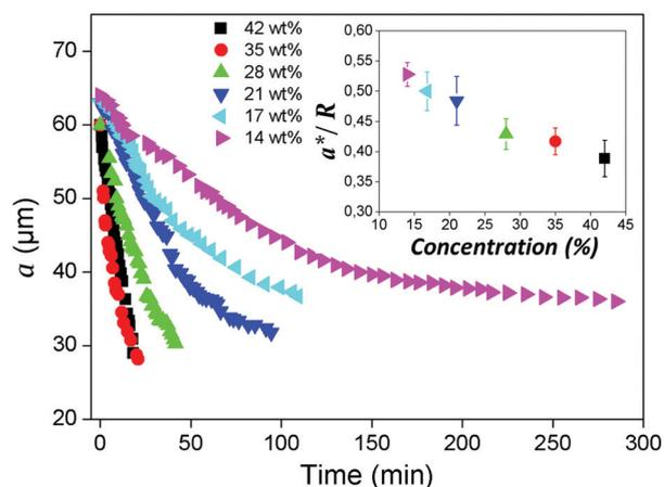
**Fig. 9** Variation of the inner droplet radius  $a$  as a function of time for different salt concentrations. Inset: Critical inner radius  $a^*$  at which the droplet is expelled as a function of salt concentration.
