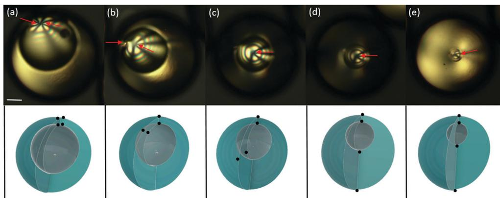
Fig. 3 (a–e) Cross-polarized images of a shell (top view) with two pairs of +1 boojums at different stages of the de-swelling process. The red arrows indicate the location of the defects. The schematics below (side view) indicate the approximate position of the two pairs of +1 boojums (black dots) for each cross-polarized image. The time scale of the de-swelling process is of the order of 10 min. Scale bar: 25  $\mu\text{m}$ .
