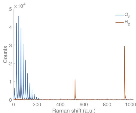
Fig. 2 Spectral signature of  $\text{O}_2$  (blue) and  $\text{H}_2$  (orange) from the Raman gas analyser.
