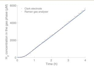
Fig. 3 Comparison between the Raman gas analyser (orange) and Clark electrodes (blue, Unisense) in real-time monitoring of  $H_2$  in the headspace of a HER. Experimental conditions: [Ir<sup>III</sup>(dF(CF<sub>3</sub>)ppy)<sub>2</sub>(-dtbbpy)]PF<sub>6</sub> (0.03 mM),<sup>17</sup> [Co<sup>II</sup>(qpy)(OH<sub>2</sub>)<sub>2</sub>](ClO<sub>4</sub>)<sup>16</sup> (0.6 mM), TEOA (0.2 M) and water (5% v/v) in acetonitrile (2 mL).
