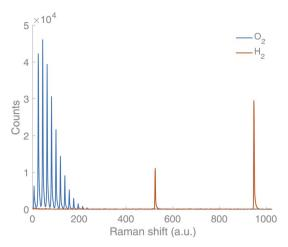
Fig. 2 Spectral signature of O<sub>2</sub> (blue) and H<sub>2</sub> (orange) from the Raman gas analyser.
