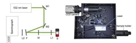
Fig. 1 Left: technical drawing of the Raman-based gas analyser. M = mirror, L = lens, F = edge filter, W = CaF<sub>2</sub> window, S = sample. Right: photo from above of the Raman gas analyser with the top cover removed.
