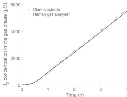
Fig. 3 Comparison between the Raman gas analyser (orange) and Clark electrodes (blue, Unisense) in real-time monitoring of  $\text{H}_2$  in the headspace of a HER. Experimental conditions:  $[\text{Ir}^{\text{III}}(\text{dF}(\text{CF}_3)\text{ppy})_2(\text{dtbbpy})]\text{PF}_6$  (0.03 mM),<sup>17</sup>  $[\text{Co}^{\text{II}}(\text{qpy})(\text{OH}_2)_2](\text{ClO}_4)$ <sup>16</sup> (0.6 mM), TEOA (0.2 M) and water (5% v/v) in acetonitrile (2 mL).
