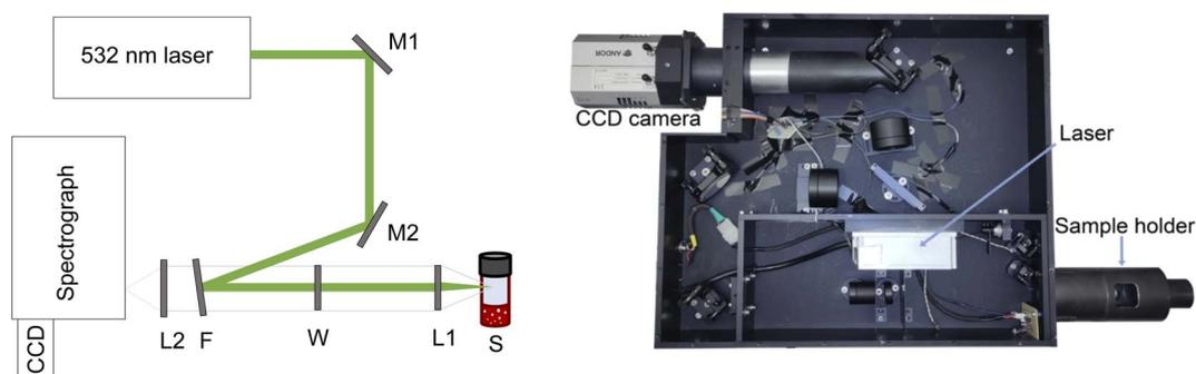
Fig. 1 Left: technical drawing of the Raman-based gas analyser. M = mirror, L = lens, F = edge filter, W =  $\text{CaF}_2$  window, S = sample. Right: photo from above of the Raman gas analyser with the top cover removed.
