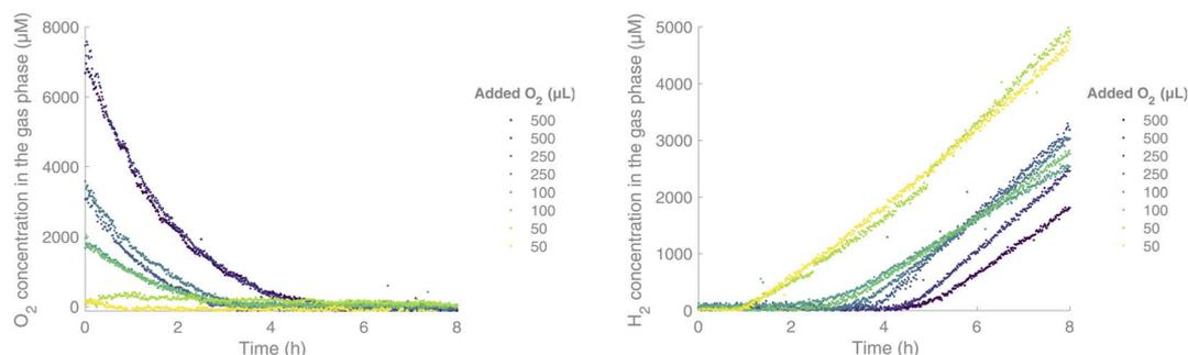
Fig. 4 Simultaneous measurement of  $O_2$  (left) and  $H_2$  (right) in a  $H_2$  formation reaction, under Ar (g) with different added amounts of  $O_2$  initially. Experimental conditions:  $[Ir^{III}(dF(CF_3)ppy)_2(dtbbpy)]PF_6$  (0.03 mM),<sup>17</sup>  $[Co^{II}(qpy)(OH_2)_2](ClO_4)^{16}$  (0.6 mM), TEOA (0.2 M) and water (5% v/v) in acetonitrile (2 mL).
