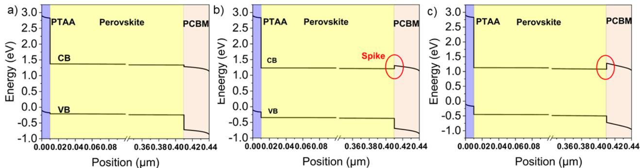
Fig. 4 Simulated energy level diagrams of PSCs based on (a) a reference perovskite with a CB minimum energy level of  $-3.85$  eV, and (b) a BiTeI-incorporating perovskite with a CB minimum energy level of  $-4.00$  eV and (c) a BiTeI-incorporating perovskite with a CB minimum energy level of  $-4.10$  eV. The energy levels are referenced to the equilibrium Fermi level in the device stack.
