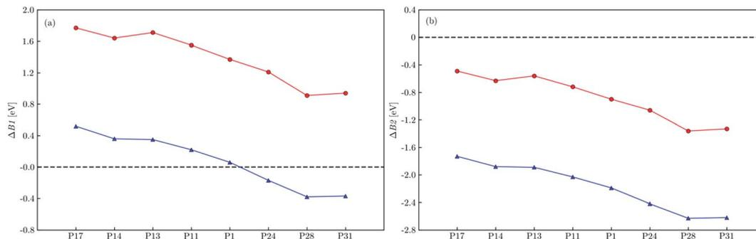
Fig. 4 The predicted free energy difference for electron transfer to the photoexcited polymer from triethylamine,  $\Delta B1$ , (a) and dehydrogenated triethylamine,  $\Delta B2$ , (b) within a dielectric continuum representing water (blue triangles) and triethylamine (red circles). All values predicted using D3-B3LYP/cc-pVTZ. See Fig. S12† for values predicted using D3-CAM-B3LYP/cc-pVTZ.
