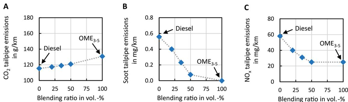
Fig. 3 (A) CO<sub>2</sub>, (B) soot, and (C) NO<sub>x</sub> tailpipe emissions of diesel-OME<sub>3-5</sub> blend combustion for various volumetric blending ratios. CO<sub>2</sub> emissions are calculated by the carbon balance for each blending ratio. Soot and NO<sub>x</sub> emissions are obtained by single-cylinder engine tests for each blending ratio, using a global design of experiments approach and subsequently simulating a complete driving cycle for a mid-size passenger car.
