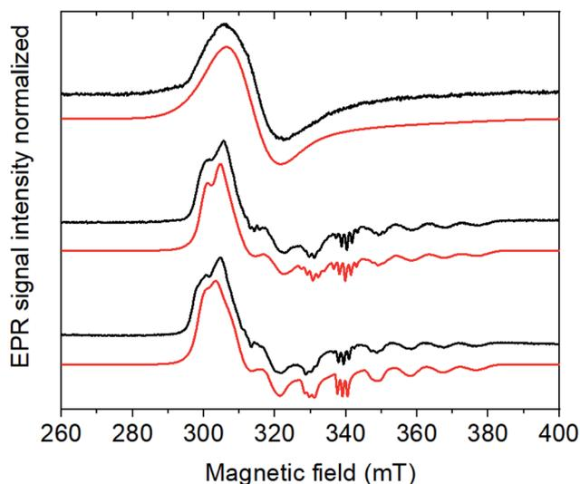
**Fig. 3** CW X-band EPR spectra (9.65 GHz) of the electrochemically generated  $\text{Co}^{\text{II}}$  form of **Cat1** (0.5 mM) as prepared (top), with 5 eq. of the acids *p*-cyanoanilinium tetrafluoroborate (middle),  $\text{HBF}_4$  (bottom) and their respective simulations in red. Experimental conditions: 30 K, 1 mW microwave power, 1600 G field sweep. Simulation parameters are reported in Table S1.†
