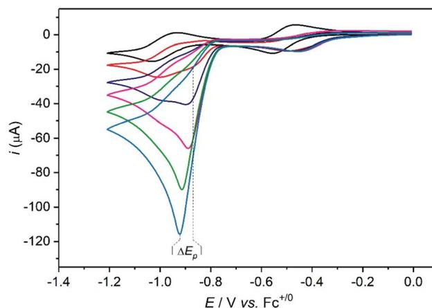
Fig. 5 Cyclic voltammograms of **Cat1** (2 mM) in  $\text{CH}_3\text{CN}$  (+0.1 M  $^t\text{Bu}_4\text{NBF}_4$ ) recorded at a glassy carbon electrode (1.6 mm diameter) in the presence of various concentrations of *p*-cyanoanilinium tetrafluoroborate at  $100 \text{ mV s}^{-1}$ : 0 (black), 4 (red), 8 (navy), 12 (magenta), 16 (green), 20 (cyan) mM.
