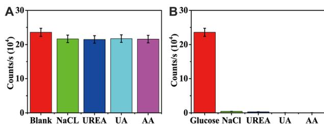
**Fig. 7** CL detection of interfering substances in 0.01 mmol L<sup>-1</sup> standard glucose solution in 5 mmol L<sup>-1</sup> solvent (A); CL detection was performed with 0.01 mmol L<sup>-1</sup> interfering substance and 5 mmol L<sup>-1</sup> glucose solution with water as solvent (B).
