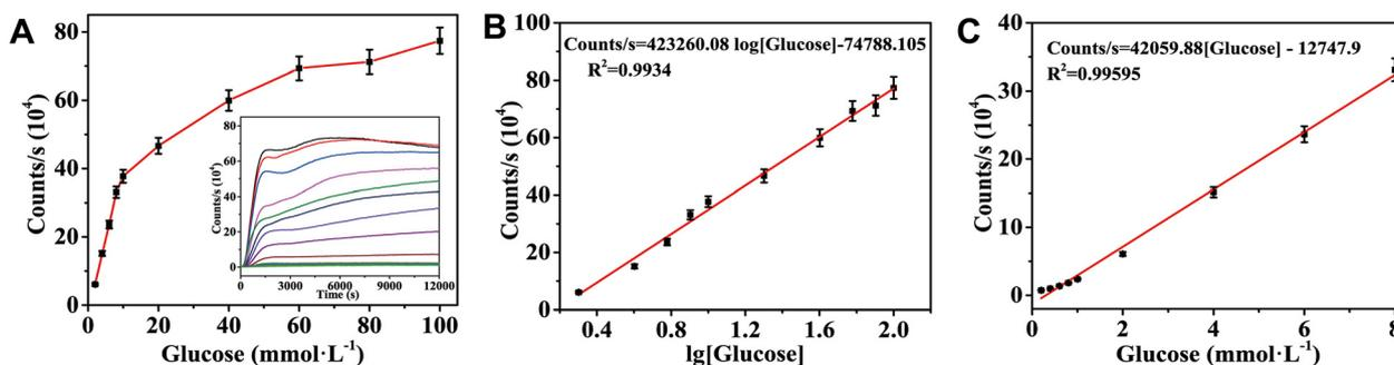
Fig. 6 The CL intensity (A) of the agarose gel system loaded with mixed materials (ZIF-67/ZIF-8@GOx/luminal) for different concentrations of glucose ranging from 0.2 to 100 mmol L<sup>-1</sup>. According to the logarithmic calibration curve (B) of CL intensity to glucose ranging from 2 to 100 mmol L<sup>-1</sup>, the error bar = relative standard deviation (RSD) ( $n = 3$ ). The linear curve of CL intensity with glucose concentration from 0.2 to 8 mmol L<sup>-1</sup> (C).
