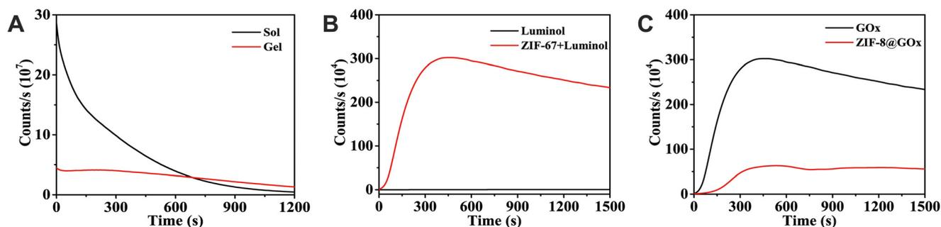
Fig. 4 Verification of the effect of 5 mmol  $\text{mL}^{-1}$   $\text{H}_2\text{O}_2$  on gel pore structure in delaying luminescence (A); validation of the catalytic effect of ZIF-67 on the  $\text{H}_2\text{O}_2$ -luminol system (B); verification of enhanced CL persistence with ZIF-8 loaded GOx (C).
