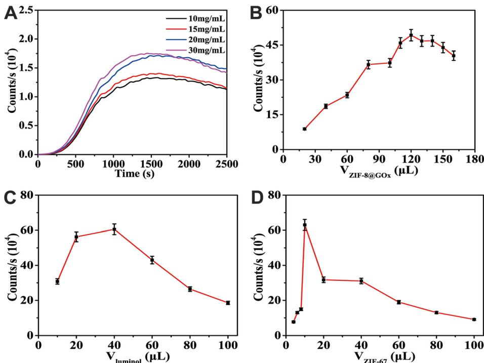
Fig. 5 Effects on CL intensity of agarose gel concentration (A), volume of the ZIF-8@GOx solution (B), volume of the luminal solution (C), volume of the ZIF-67 solution (D) for detecting 20 mg mL<sup>-1</sup> glucose solution.
