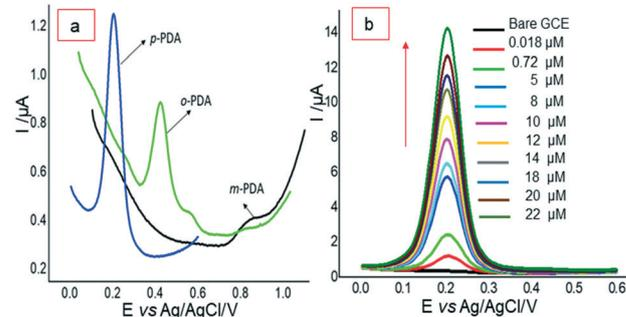
Fig. 4 (a) DPVs for electrocatalytic oxidation of *p*-PDA, *o*-PDA and *m*-PDA on IL-GO@Cu-Ag/GCE at different potentials. (b) DPVs of *p*-PDA oxidation with different concentrations. Reproduced from ref. 65 with permission from Elsevier, copyright 2021.
