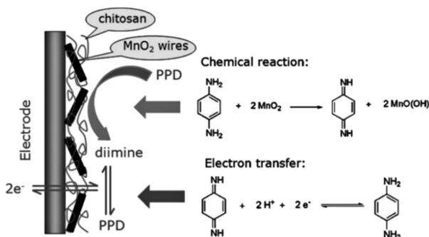
**Fig. 2** The chemical–electrochemical process of *p*-PDA on  $\beta$ -MnO<sub>2</sub> nanowire/GCE. Reproduced from ref. 57 with permission from John Wiley and Sons, copyright 2010.
