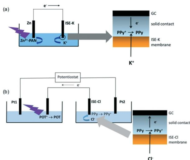
**Fig. 6** Schemes of the reported bipolar ISE systems to convert potential to the fluorescence change of POT (a) or for the fluorescence determination of zinc ion concentration change. Adapted from ref. 73 and 74. Copyright: Wiley-VCH and Elsevier, respectively.
