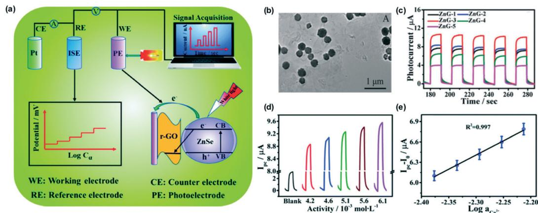
**Fig. 7** (a): An illustration of the PEC sensing platform to read the potentiometric response of an ISE. (b): TEM image of the as-prepared ZnSe/r-GO. (c): Time traces of the photocurrent responses of ZnG-1, 2, 3, 4, and 5 composite photoelectrodes at a potential of 0.25 V. (d): Photocurrent responses of the ZnSe/r-GO modified GE electrodes with variable calcium activities from 4.2 to 6.1 mM. (e): Corresponding calibration curve. Adapted from ref. 75. Copyright: Royal Society of Chemistry.
