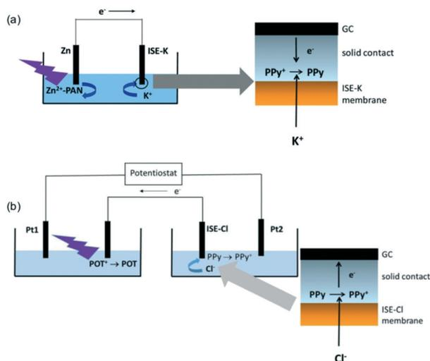
**Fig. 6** Schemes of the reported bipolar ISE systems to convert potential to the fluorescence change of POT (a) or for the fluorescence determination of zinc ion concentration change. Adapted from ref. 73 and 74. Copyright: Wiley-VCH and Elsevier, respectively.
