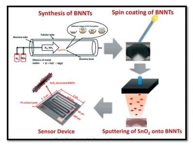
Fig. 8 The schematic of the flow process for the SnO<sub>2</sub>-BNNTs sensor. <sup>173</sup>
