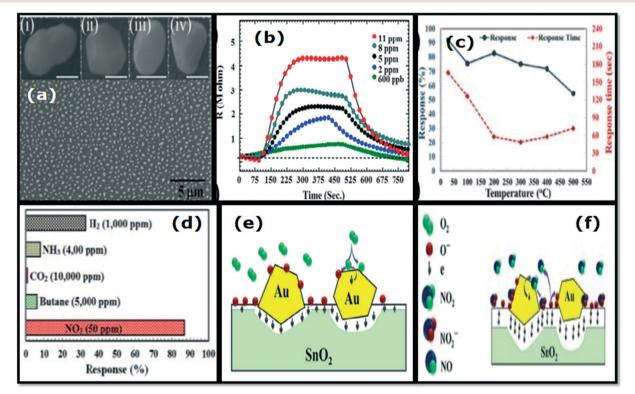
Fig. 6 (a) SEM image of the Au/SnO<sub>2</sub> thin film, (b) response-recovery curves of the Au/SnO<sub>2</sub> sensor in various concentrations of NO<sub>2</sub>, (c) response and response time at different operating temperatures, (d) selectivity of the fabricated sensor for various target gases, and (e and f) the schematics of the sensing mechanism. 113
