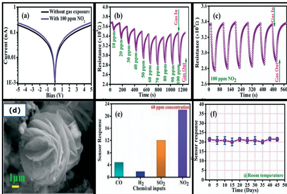
Fig. 7 (a) Log scale I-V curves. Resistance response during cyclic exposure at (b) different and (c) fixed concentrations. Sensor response versus (d)  $\text{Co}_3\text{O}_4$  FESEM and (e) different chemical inputs, and (f) stability of the sensor at RT.<sup>105</sup>
