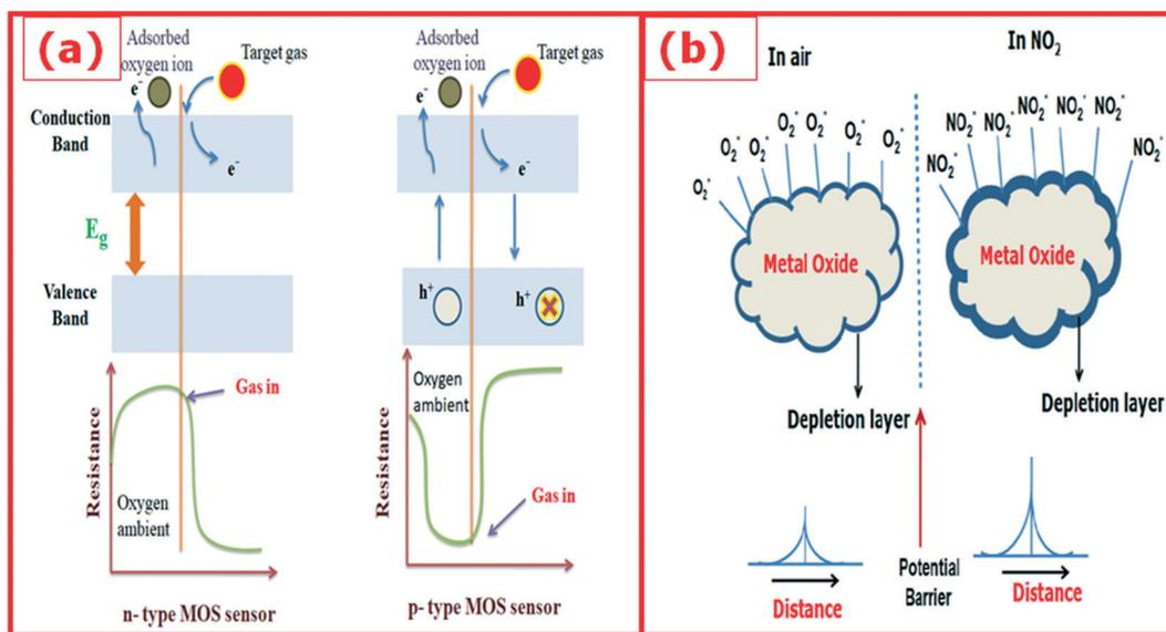
Fig. 5 (a) Schematic diagram: sensing mechanism of n-type and p-type MOSs. (b) The interaction of oxygen and NO<sub>2</sub> with n-type semiconducting metal oxides. Charge distribution following the adsorption of oxygen (left) and NO<sub>2</sub> (right) on the surface of the metal oxide. The resulting potential distribution across the grain boundaries is also shown in the figure.
