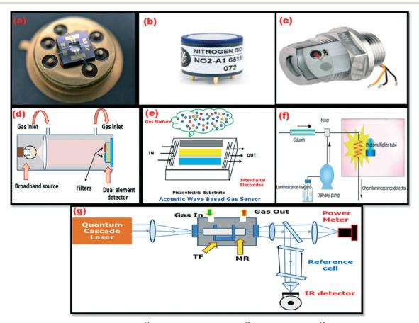
Fig. 4 Different NO<sub>2</sub> gas sensors: (a) MOS sensor, <sup>44</sup> (b) electrochemical sensor, <sup>45</sup> (c) catalytic sensor, <sup>46</sup> (d) optical sensor, (e) acoustic wave sensor, (f) chemiluminescence and (g) photoacoustic spectroscopy.
