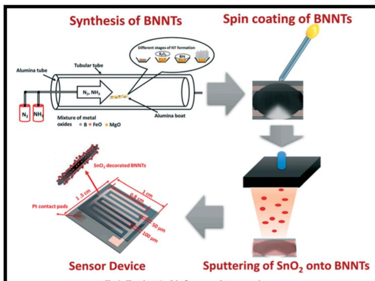
Fig. 8 The schematic of the flow process for the  $\text{SnO}_2$ -BNNTs sensor.<sup>173</sup>
