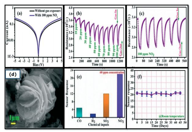
Fig. 7 (a) Log scale I-V curves. Resistance response during cyclic exposure at (b) different and (c) fixed concentrations. Sensor response versus (d) Co<sub>3</sub>O<sub>4</sub> FESEM and (e) different chemical inputs, and (f) stability of the sensor at RT. 105
