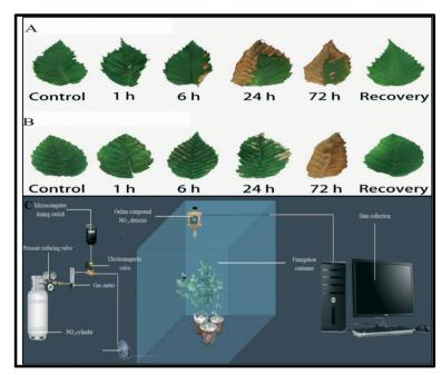
Fig. 2 Leaves of (A) Carpinus betulus (B) and Carpinus putoens showing injury symptoms under different NO2 exposure times and after natural recovery. (c) The experimental set-up for timing regulation and recording of NO<sub>2</sub> concentration.<sup>27</sup>
