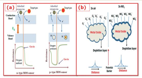
Fig. 5 (a) Schematic diagram: sensing mechanism of n-type and p-type MOSs. (b) The interaction of oxygen and NO<sub>2</sub> with n-type semiconducting metal oxides. Charge distribution following the adsorption of oxygen (left) and NO2 (right) on the surface of the metal oxide. The resulting potential distribution across the grain boundaries is also shown in the figure.
