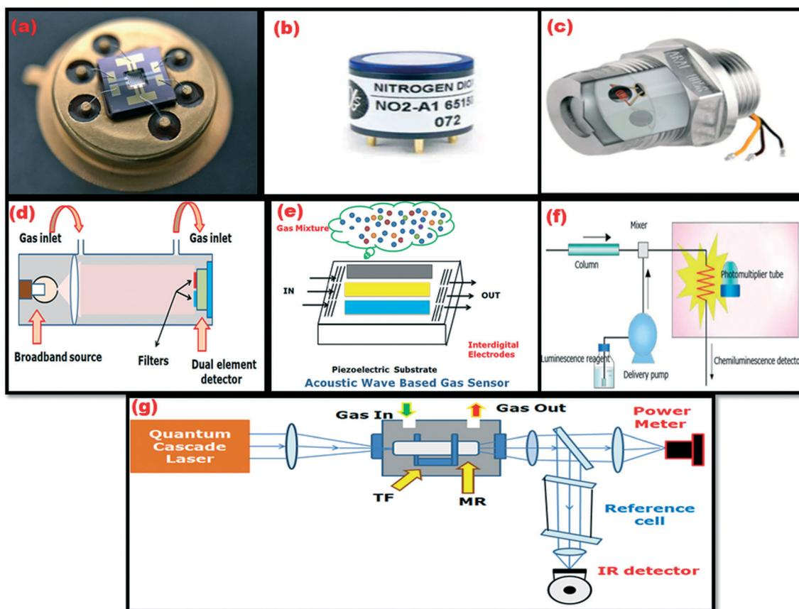
Fig. 4 Different  $\text{NO}_2$  gas sensors: (a) MOS sensor,<sup>44</sup> (b) electrochemical sensor,<sup>45</sup> (c) catalytic sensor,<sup>46</sup> (d) optical sensor, (e) acoustic wave sensor, (f) chemiluminescence and (g) photoacoustic spectroscopy.
