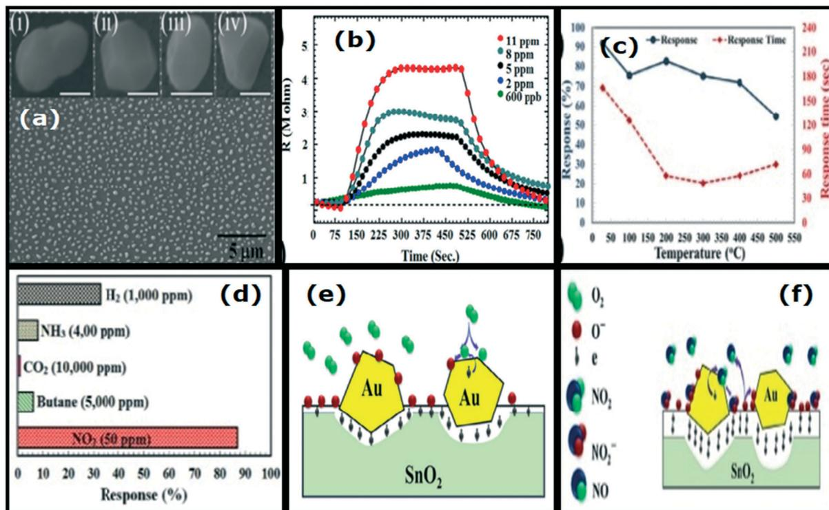
Fig. 6 (a) SEM image of the Au/ $\text{SnO}_2$  thin film, (b) response-recovery curves of the Au/ $\text{SnO}_2$  sensor in various concentrations of  $\text{NO}_2$ , (c) response and response time at different operating temperatures, (d) selectivity of the fabricated sensor for various target gases, and (e and f) the schematics of the sensing mechanism.<sup>113</sup>
