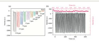
Fig. 3 (a) Signal intensity of the nanomesh scaffold-modified sensor recorded at different pyridine concentrations (varying from 4.8 ppb to 3750 ppm, 25 °C); (b) reusability and photochemical stability test of the nanomesh scaffold-modified sensor towards pyridine vapor ( $c_{pyridine}$  = 3750 ppm, 25 °C).
