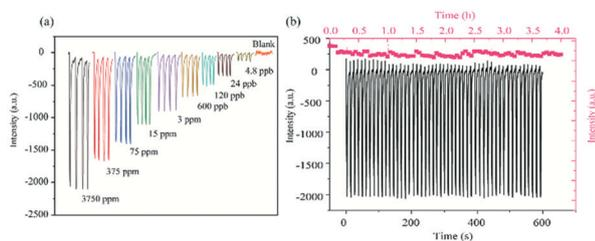
**Fig. 3** (a) Signal intensity of the nanomesh scaffold-modified sensor recorded at different pyridine concentrations (varying from 4.8 ppb to 3750 ppm, 25 °C); (b) reusability and photochemical stability test of the nanomesh scaffold-modified sensor towards pyridine vapor ( $c_{\text{pyridine}} = 3750$  ppm, 25 °C).
