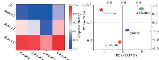
**Fig. 4** (a) Hot plot of the response intensity of three sensors on exposure to pyridine and its derivatives (2-picoline, 3-picoline and 4-picoline), sensor 1 and sensor 2 was based on the nanomesh scaffold-modified substrate with 300 nm and 200 nm hole depths, sensor 3 was based on the ground glass substrate. (b) Two-dimensional PCA score plot for discriminating the saturated vapor of pyridine and its derivatives at 293 K via utilization of the response intensity of three sensors.
