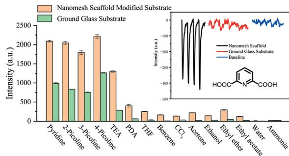
**Fig. 2** Selectivity tests of the nanomesh scaffold-modified sensor and ground glass-based sensor to various pyridine derivatives and common solvent vapors. THF = tetrahydrofuran. Inset: the response intensity of the nanomesh scaffold-modified sensor and ground glass-based sensor towards saturated 2,6-dicarboxyridine vapor conducted at 25 °C.
