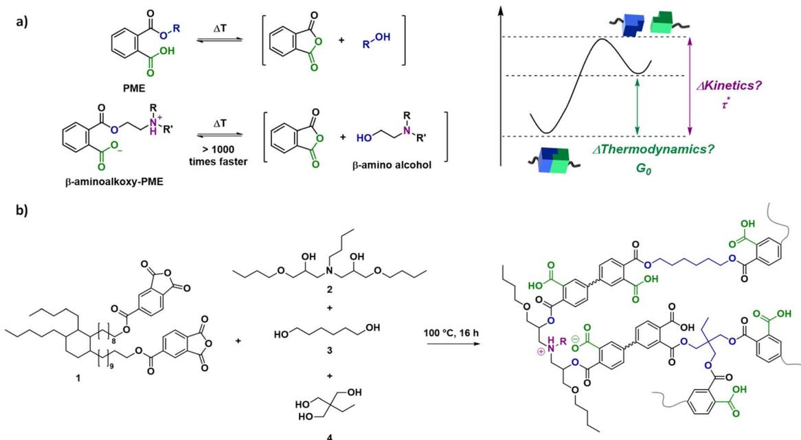
Scheme 1 Schematic representation of the model system used, highlighting the transesterification of phthalate monoesters (PMEs) with two cross-links of varying reactivity.<sup>20</sup> (a) Scheme for dissociation reaction of a phthalate monoester with and without substituents on the  $\beta$ -carbon. (b) Network synthesis by mixing a dianhydride and polyol mixture.
