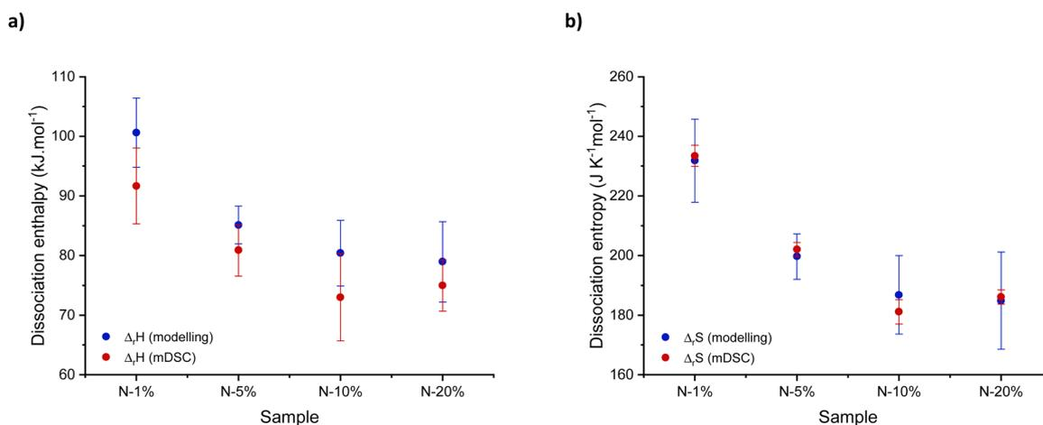
Fig. 6 Overview of obtained (a) dissociation enthalpy ( $\Delta H$ ) and (b) entropy ( $\Delta S$ ) values after modelling of rheology data and temperature-modulated differential scanning calorimetry (mDSC) analysis.
