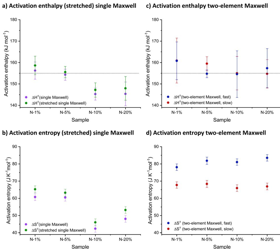
Fig. 3 Overview of obtained activation enthalpy ( $\Delta H^\ddagger$ ) and activation entropy ( $\Delta S^\ddagger$ ) values after Eyring analysis of rheology data using a single (stretched) exponential fit for (a) and (b) or a double exponential fit for (c) and (d).
