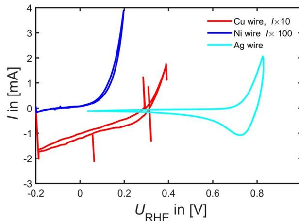
Fig. 6 FAOR data on a Cu, Ni and Ag wire at 50 mV s<sup>-1</sup> at room-temperature Ar-saturated 0.1 M HClO<sub>4</sub> with 0.1 M HCOOH taken at 50 mV s<sup>-1</sup>.
