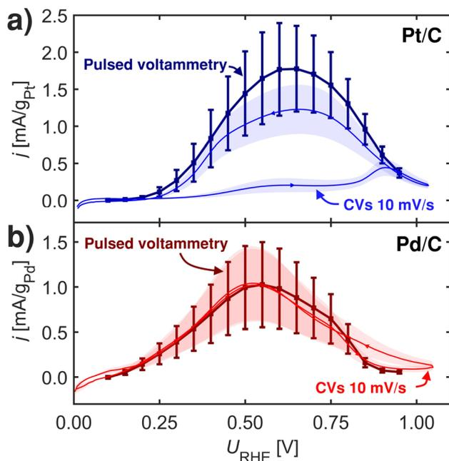
Fig. 5 2 s pulsed voltammetry and CVs at  $10 \text{ mV s}^{-1}$  at room-temperature at 1600 rpm in Ar-saturated 0.1 M  $\text{HClO}_4$  with 0.1 M  $\text{HCOOH}$ . (a) Pt/C. (b) Pd/C. Measurements repeated three times.
