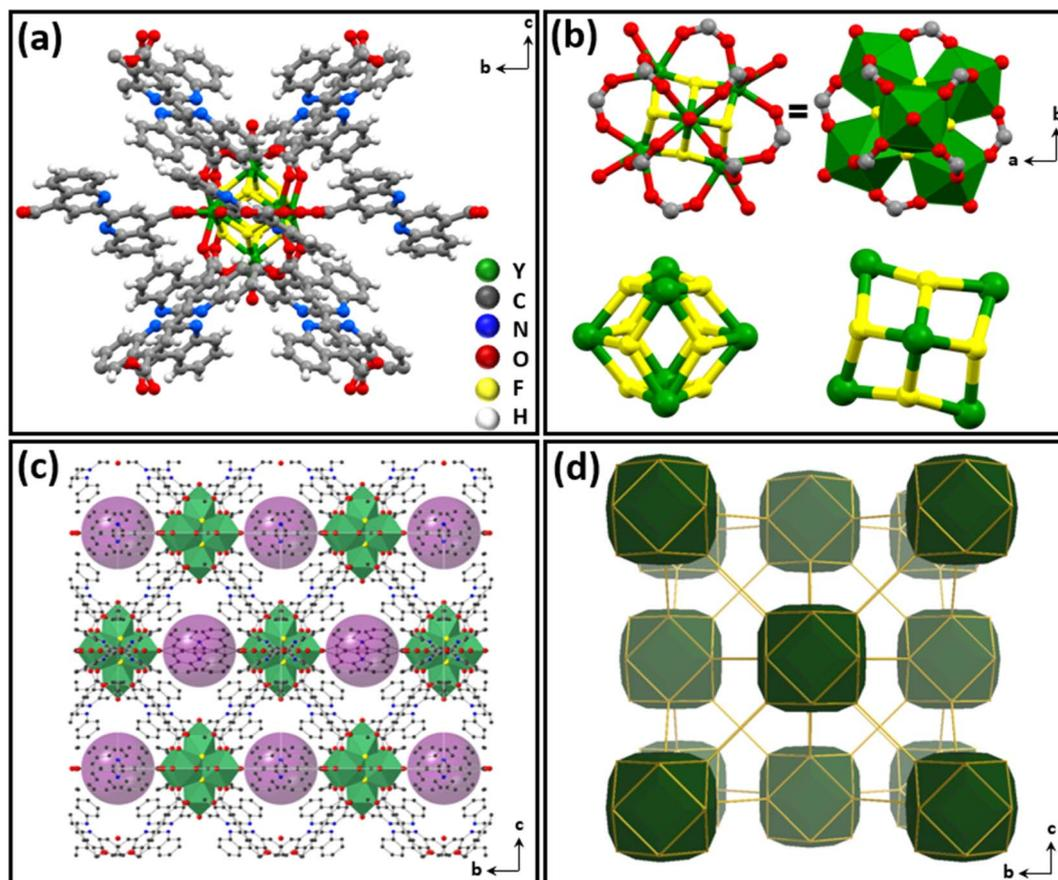
Fig. 4 Crystal structure of Y-BCA-3D (a) cluster structure with hexanuclear node, (b) c-axis view of hexacluster and isolated Y<sub>6</sub>F<sub>8</sub> cluster, (c) extended 3D network view along the a-axis showing 6.3 Å spherical cavities (purple), and (d) underlying net topology of the MOF viewed along the a-axis.
