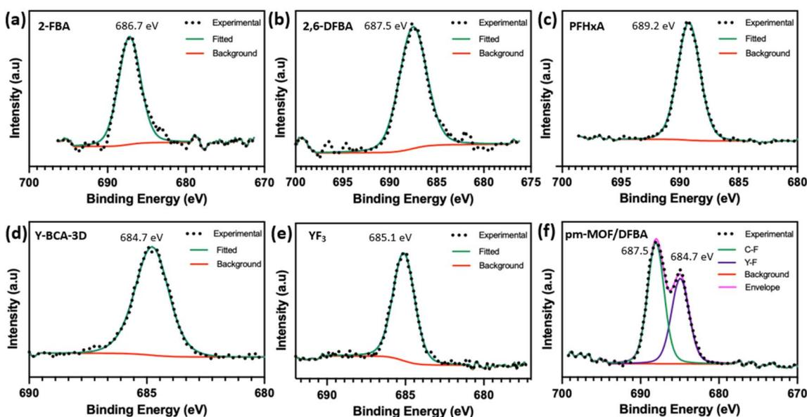
Fig. 6 High resolution F 1s XPS spectra of (a) 2-FBA, (b) 2,6-DFBA, (c) PFHxA, (d) Y-BCA-3D, (e) YF<sub>3</sub>, and (f) physical mixture of Y-BCA-3D and 2,6-DFBA.
