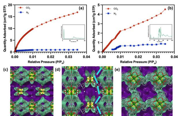
Fig. 7 Adsorption isotherms for (a) Y-BCA-3D and (b) Y-BCA-2D. Representation of sinusoidal voids/channels (purple) in Y-BCA-3D (c) viewed along  $a$ -axis, (d) viewed along  $b$ -axis and gas passage is highlighted by arrows, and (e) viewed along  $c$ -axis show presence of deep spherical cavities with a diameter of 6.3 Å.
