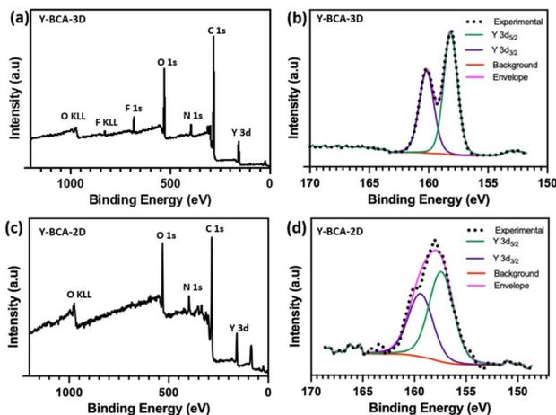
Fig. 5 The XPS spectra of (a) Y-BCA-3D survey, (b) Y-BCA-3D high resolution Y 3d<sub>5/2</sub> and 3d<sub>3/2</sub>, (c) Y-BCA-2D survey, and (d) Y-BCA-2D high resolution Y 3d<sub>5/2</sub> and 3d<sub>3/2</sub>.
