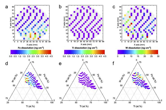
Fig. 2 Element-specific dissolution of Fe-Ti-W-O material library at 1.7 V<sub>RHE</sub>. (a-c) Dissolved amounts of Fe (a), Ti (b), and W (c) mapped onto a schematic representation of the wafer. (d-f) Dissolved amounts of Fe (d), Ti (e), and W (f) mapped onto a ternary diagram. The HT measurements were conducted in 0.05 M NaNO<sub>3</sub> (pH 5.7) under 1 Sun Am 1.5G illumination. Note that the color scale for W differs from Fe and Ti.
