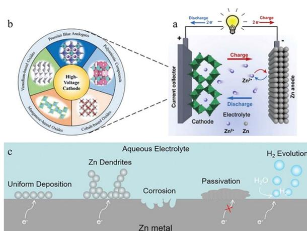
Fig. 1 (a) Schematic illustration of the working principle of ZIBs. Adapted from ref. 11. Copyright 2020, *Chem. Soc. Rev.* (b) Representative cathode materials. Adapted from ref. 16. Copyright 2021, Wiley-VCH. (c) Schematic diagram of interactions with aqueous electrolyte on the zinc anode surface.
