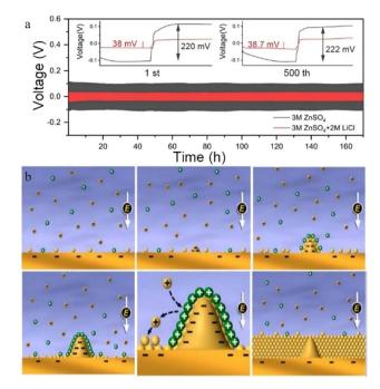
Fig. 7 (a) Galvanostatic charge—discharge curves in different electrolytes. Adapted from ref. 100. Copyright 2021, American Chemical Society. (b) The self-healing electrostatic shield mechanism. Adapted from ref. 102. Copyright 2013, American Chemical Society.
