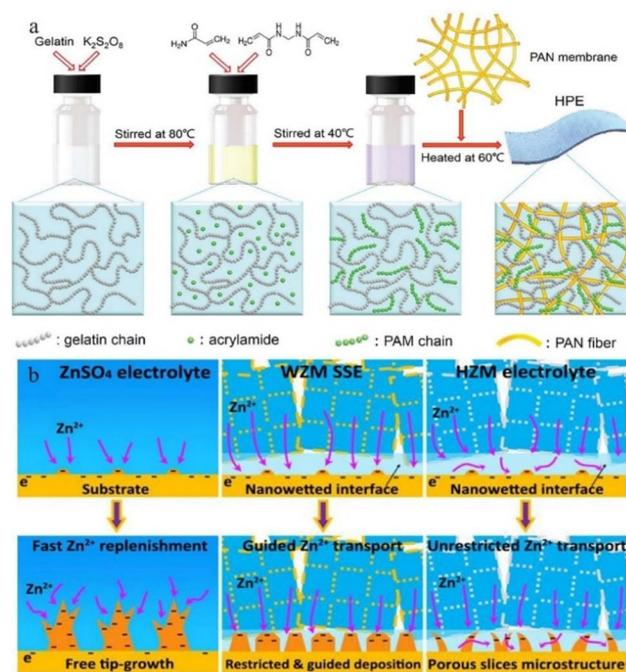
Fig. 13 (a) Synthesis of HPE. Adapted from ref. 135. Copyright 2018, Royal Society of Chemistry. (b) Mechanisms of deposition behaviours of ZnSO<sub>4</sub> electrolytes, water@ZnMOF-808-solid-state electrolyte (WZM), and hybrid ZnSO<sub>4</sub>@MOF-808 (HZM) electrolyte. Adapted from ref. 143. Copyright 2018 Elsevier Ltd.
