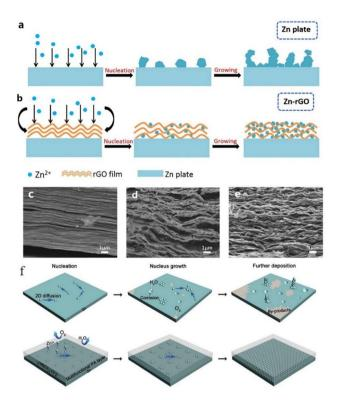
Fig. 15 Zn deposition process on (a) the unprocessed Zn anode and (b) Zn-rGO anode. SEM images of rGO coating (c) before cycling and (d and e) after cycling. Adapted from ref. 150. Copyright 2019, Elsevier. (f) Zn plating process with PA coating. Adapted from ref. 151. Copyright 2019, The Royal Society of Chemistry.
