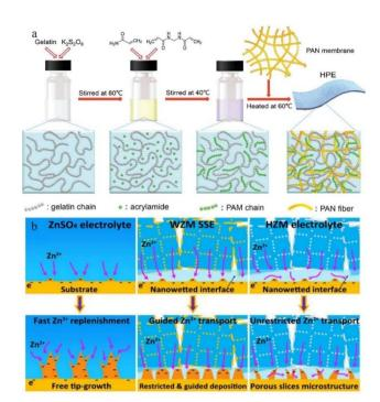
Fig. 13 (a) Synthesis of HPE. Adapted from ref. 135. Copyright 2018, Royal Society of Chemistry. (b) Mechanisms of deposition behaviours of  $ZnSO_4$  electrolytes, water@ZnMOF-808-solid-state electrolyte (WZM), and hybrid  $ZnSO_4$ @MOF-808 (HZM) electrolyte. Adapted from ref. 143. Copyright 2018 Elsevier Ltd.
