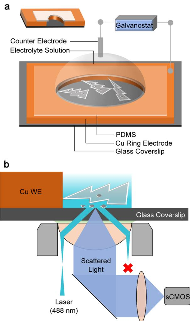
Fig. 1 Schematic illustration of the experimental setup. (a) A model zinc air battery with the cross-section view of the cell in the upper-left corner (electrochemical setup) and (b) *in situ* TIRDFM (reflected light is rejected)-based set-up used to collect scattered light during the zinc-plating process.
