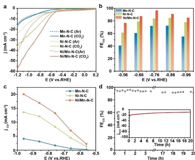
Fig. 3 (a) LSV curves performed in Ar-saturated and CO<sub>2</sub>-saturated 0.5 M KHCO<sub>3</sub> solution of Ni/Mn–N–C, Ni–N–C, and Mn–N–C; (b) potential-dependent FE<sub>CO</sub>, (c) potential-dependent *j*<sub>CO</sub> of the Ni/Mn–N–C, Ni–N–C and Mn–N–C catalyst for CO<sub>2</sub>RR, (d) long-term stability of Ni/Mn–N–C for CO<sub>2</sub>RR at –0.76 V.
