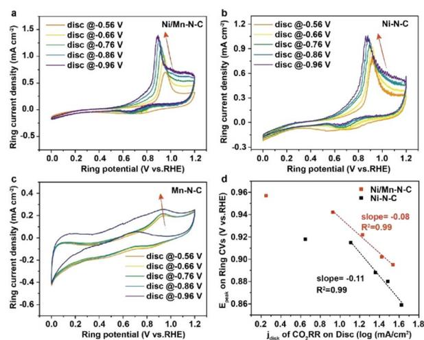
Fig. 4 Cyclic voltammograms of CO oxidation on Pt ring electrode on the (a) Ni/Mn–N–C, (b) Ni–N–C, (c) Mn–N–C disk electrode under different CO<sub>2</sub>RR potentials, (d) the dependence of CO oxidation peak potential on the log value of electrolysis current for Ni/Mn–N–C and Ni–N–C catalysts.
