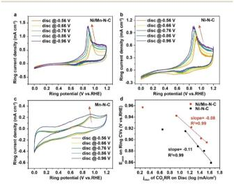
Fig. 4 Cyclic voltammograms of CO oxidation on Pt ring electrode on the (a) Ni/Mn–N–C, (b) Ni–N–C, (c) Mn–N–C disk electrode under different  $CO_2RR$  potentials, (d) the dependence of CO oxidation peak potential on the log value of electrolysis current for Ni/Mn–N–C and Ni–N–C catalysts.
