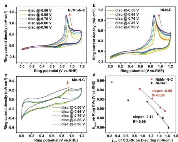
Fig. 4 Cyclic voltammograms of CO oxidation on Pt ring electrode on the (a) Ni/Mn–N–C, (b) Ni–N–C, (c) Mn–N–C disk electrode under different CO<sub>2</sub>RR potentials, (d) the dependence of CO oxidation peak potential on the log value of electrolysis current for Ni/Mn–N–C and Ni–N–C catalysts.
