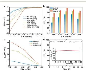
Fig. 3 (a) LSV curves performed in Ar-saturated and CO<sub>2</sub>-saturated 0.5 M KHCO<sub>3</sub> solution of Ni/Mn–N–C, Ni–N–C, and Mn–N–C; (b) potential-dependent FE<sub>CO</sub>, (c) potential-dependent  $j_{CO}$  of the Ni/Mn–N–C, Ni–N–C and Mn–N–C catalyst for CO<sub>2</sub>RR, (d) long-term stability of Ni/Mn–N–C for CO<sub>2</sub>RR at -0.76 V.
