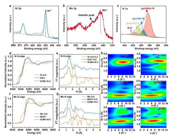
Fig. 2 (a) The Ni 2p XPS spectra, (b) the Mn 2p XPS spectra, (c) the high-resolution N 1s XPS spectra, (d) Ni K edge XANES spectra, (e) Ni K edge EXAFS spectra, (f) Mn K edge XANES spectra, (g) Mn K edge EXAFS spectra of Ni/Mn-N-C, (h) wavelet transform of the  $k^3$ -weighted Ni K edge and Mn K edge EXAFS data of Ni/Mn-N-C and reference samples (Ni foil, NiPc, Mn foil and MnPc).
