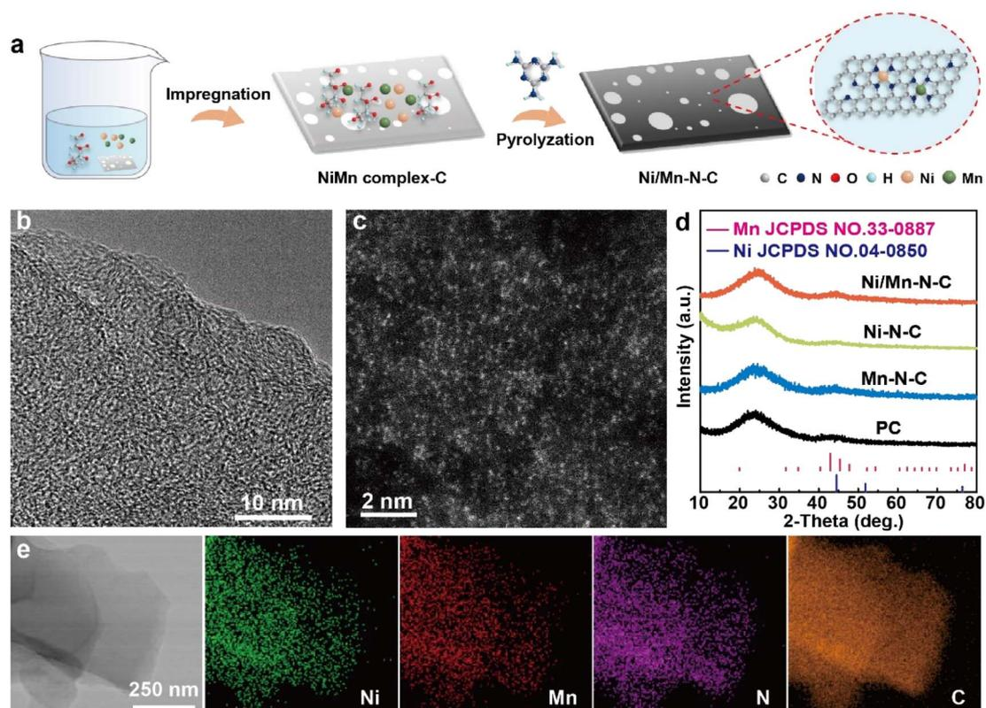
Fig. 1 (a) Scheme for the synthesis of Ni/Mn-N-C catalyst, (b) HRTEM image, (c) HAADF-STEM image, (d) XRD patterns, and (e) TEM and corresponding elemental mapping images of Ni/Mn-N-C catalyst.
