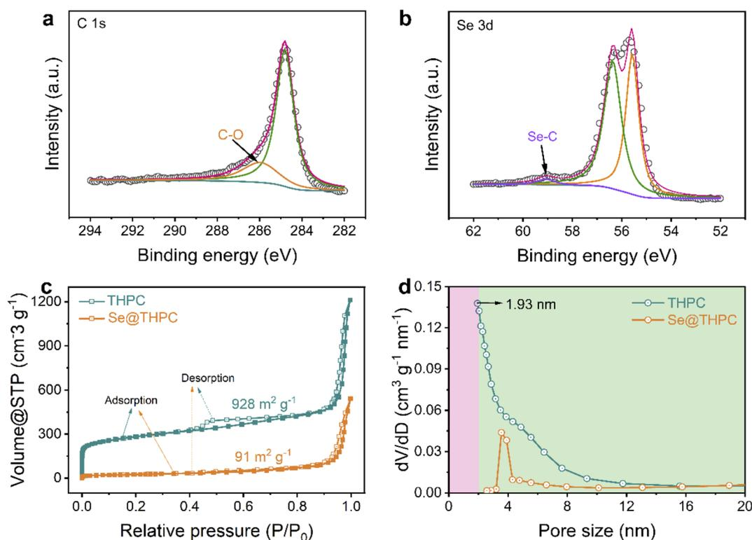
Fig. 3 XPS spectra of C 1s (a) and Se 3d (b); N<sub>2</sub> adsorption–desorption isotherms (c) and pore-size distribution (d) of the THPC and Se@THPC composite.
