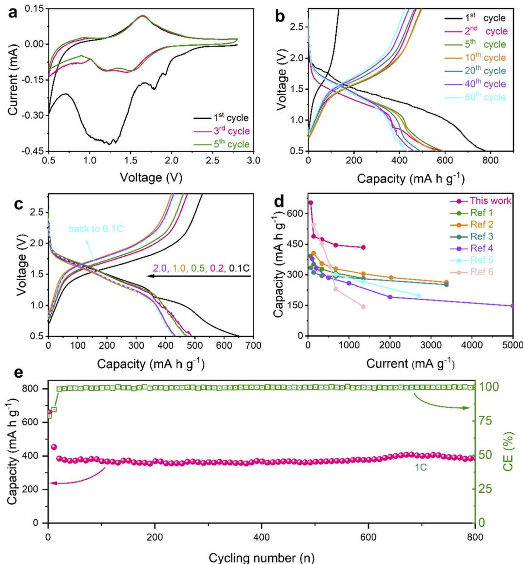
Fig. 4 Electrochemical performance of the Se@THPC composite. (a) CV curves at a scan rate of  $0.1 \text{ mV s}^{-1}$ ; (b) discharge–charge profiles at  $0.1\text{C}$ ; (c) discharge–charge profiles at various rates; (d) a comparison of rate capabilities between this work and other studies (ref. 1–6 are provided in the ESI†); (e) prolonged cycling stability at  $1\text{C}$ .
