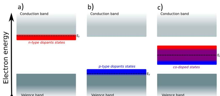
**Fig. 2** (a) Insertion of an n-type dopant in a semiconductor, (b) insertion of a p-type dopant in a semiconductor, (c) simultaneous insertion of an n-type and a p-type dopant in a semiconductor and the creation of the compensated electron states.
