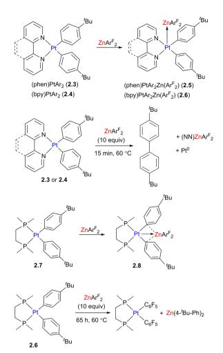
Scheme 5 The structure and reactivity of Pt/Zn complexes as a function of the supporting ligand on Pt.
