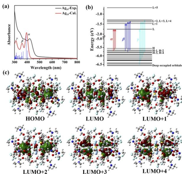
Fig. 4 UV-vis absorption spectra and DFT of  $\text{Ag}_{24}$ . (a) Experimental (black) and calculated (red) absorption spectra of  $\text{Ag}_{24}$  in  $\text{CH}_2\text{Cl}_2$ . (b) The Kohn–Sham orbital energy level of  $\text{Ag}_{24}$ . (c) Frontier orbitals including HOMO, LUMO, LUMO+1, LUMO+2, LUMO+3 and LUMO+4 of  $\text{Ag}_{24}$ .
