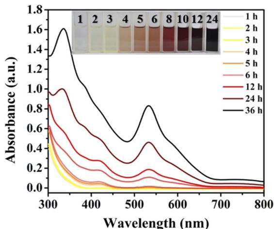
Fig. 1 Time-dependent UV-vis absorption spectra for tracking the reaction process. Experimental method: 9 mg  $\{Ag(S^iPr)_n\}$ , 22 mg  $CF_3COOAg$ , and 50  $\mu L$   $CF_3COOH$  in the solvent mixture (iPrOH : DMF = 3 : 1) at 80  $^\circ C$ . Inset: the colour of mother liquor after the solvothermal reaction at different times (1–24 h).
