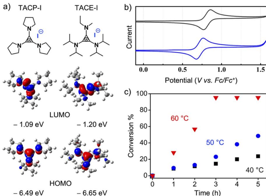
Fig. 3 (a) The chemical structures and the calculated frontier molecular orbitals of TACP-I and TACE-I; (b) cyclic voltammograms of TACP-PF<sub>6</sub> (blue) and TACE-PF<sub>6</sub> (black), Fc/Fc<sup>+</sup>: ferrocene/ferrocenium; (c) the time-conversion plot of the radical trapping catalyzed by TACE-I.
