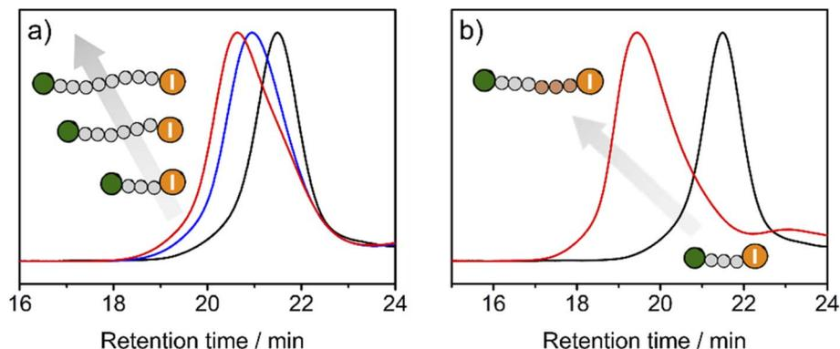
Fig. 5 The GPC chromatograms of chain-extension polymerization (0 min: black; 40 min: blue; 60 min: red) and block polymerization (macroinitiator: black; PMMA-*b*-PBzMA: red). Characterized using GPC with DMF as eluent and PMMA as standard.
