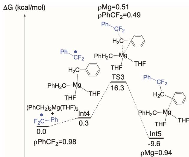
Fig. 7 Computed C–C coupling pathway at  $\text{MgBn}_2(\text{THF})_2$ .
