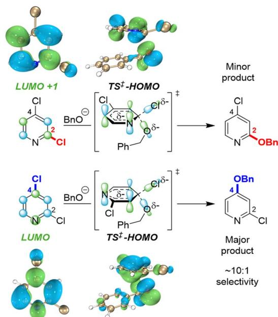
Fig. 6 FMO analysis of S<sub>N</sub>Ar selectivity with 2,4-dichloropyridine, revealing orbital symmetry effects in the substrate (LUMO versus LUMO+1) and transition states (HOMO contributions from *ortho* and *para* sites).
