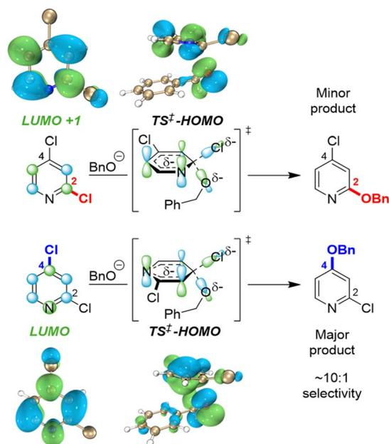
Fig. 6 FMO analysis of  $\text{S}_{\text{N}}\text{Ar}$  selectivity with 2,4-dichloropyridine, revealing orbital symmetry effects in the substrate (LUMO versus LUMO+1) and transition states (HOMO contributions from *ortho* and *para* sites).
