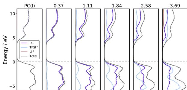
Fig. 2 Projected electronic density of states (PDOS) of PC solutions with LiTFSI concentrations of 0, 0.37, 1.11, 1.84, 2.58 and 3.69 mol L<sup>-1</sup>. They are averaged every 50 fs along AIMD trajectories of the last 10 ps. The functional used is BLYP.
