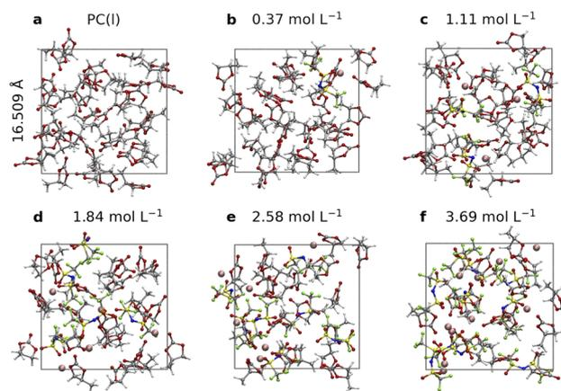
Fig. 1 Simulation supercells of (a) liquid PC and PC with (b) 0.37, (c) 1.11, (d) 1.84, (e) 2.58 and (f) 3.69 mol L<sup>−1</sup> LiTFSI. These six configurations are snapshots taken from AIMD trajectories. The C, H, O, N, S, F and Li atoms are in gray, white, red, blue, yellow, green and pink, respectively.
