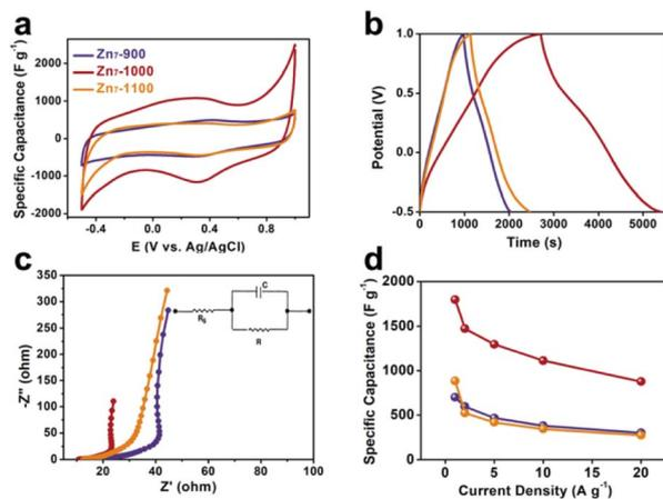
Fig. 3 Supercapacitive performance of **Zn<sub>7</sub>-Ts**. (a) A comparison of the CV curves at  $5$   $\text{mV s}^{-1}$ . (b) A comparison of the GCD curves at a current density of  $1$   $\text{A g}^{-1}$ . (c) A comparison of the electrochemical impedance spectroscopy (EIS) data. (d) A comparison of the specific capacitance values of **Zn<sub>7</sub>-900**, **Zn<sub>7</sub>-1000**, and **Zn<sub>7</sub>-1100**.
