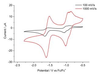
Fig. 5 Cyclic voltammetry plots for  $5^{Cy}$  at a scan rate of 100 mV s<sup>-1</sup> and 1000 mV s<sup>-1</sup> in acetonitrile (0.1 M [ $nBu_4N$ ][PF<sub>6</sub>]).
