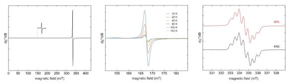
Fig. 2 CW EPR spectrum of  $6^{Cy}$  in a 1 : 1 toluene/acetonitrile mixture at 40 K (left), temperature dependence of the half-field transitions between 10 and 140 K (middle), and experimental (black) and simulated (red) EPR spectra of  $7^{Cy}$  in acetonitrile (right). Best-fit simulation parameters:  $g_{iso} = 2.0029$ ,  $a_i^{14}N_i = 14.2$  MHz (1N), 11.8 MHz (2N), and  $a_i^{1}N_i = 3.2$  MHz (6H).
