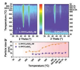
Fig. 1 (a) In situ XRD patterns of  $0.1Pt7Cu/SiO_2-IM$  and  $0.1Pt7CuSiO_3$  under a reductive atmosphere. (b) The evolution of the size of PtCu NPs versus temperature for reduction of  $0.1Pt7Cu/SiO_2-IM$  and  $0.1Pt7CuSiO_3$  in 10 vol%  $H_2/Ar$ .
